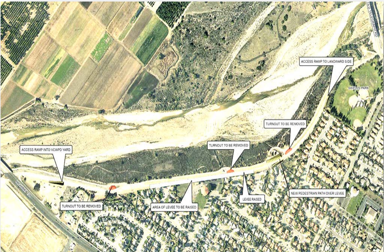
Figure 1 – Sespe Creek Levee: Location of Proposed Modifications
