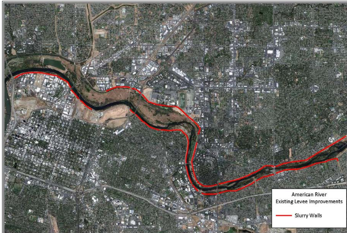
Figure 2-11: Existing Levee Improvements on the American River authorized by WRDA 96 and 99.
