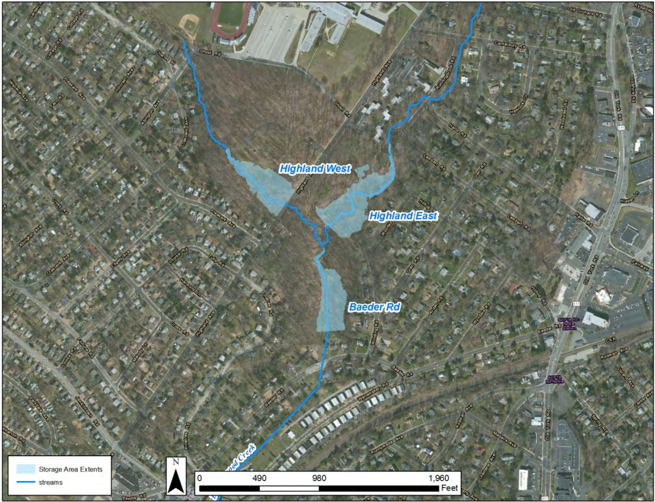
Figure 5. A close up of three of the areas being considered for dry detention basins.
