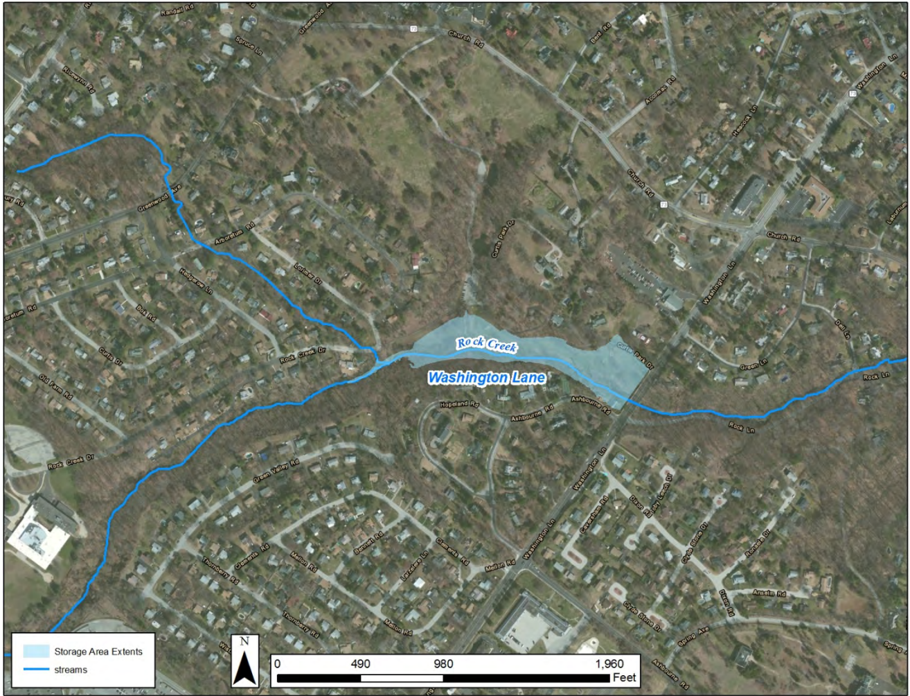
Figure 6. A close up of the Washington Lane area being considered for a dry detention basin.
