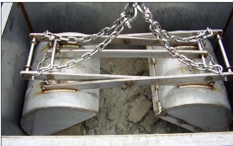
Custom Petersen-style grab sampler with sediment inside a stainless steel bin
