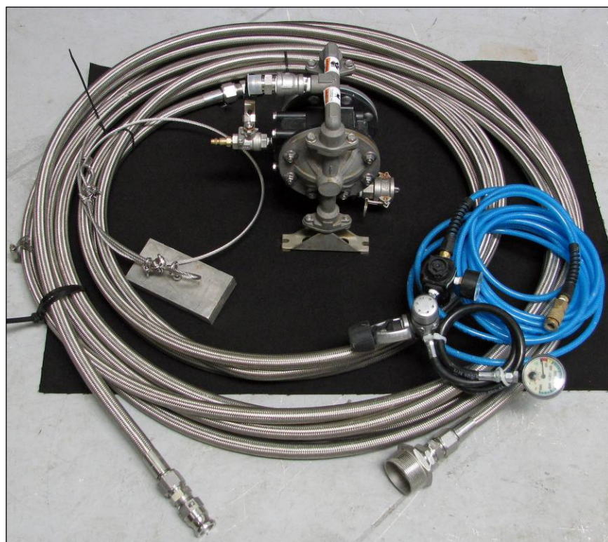
Pneumatic water pump with regulator, pressurized air tubing, weight, and stainless steel-encased Teflon ® hoses
