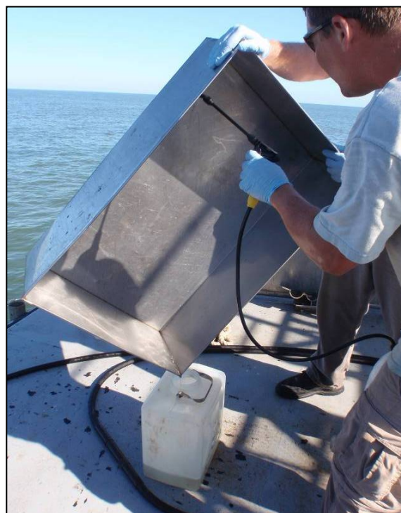
Decontaminating a stainless steel bin
