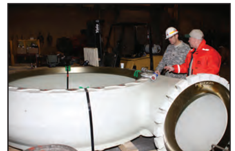
Pat Chambers discusses with Col Eckstein the new pump housing to be placed in the Dredge.
