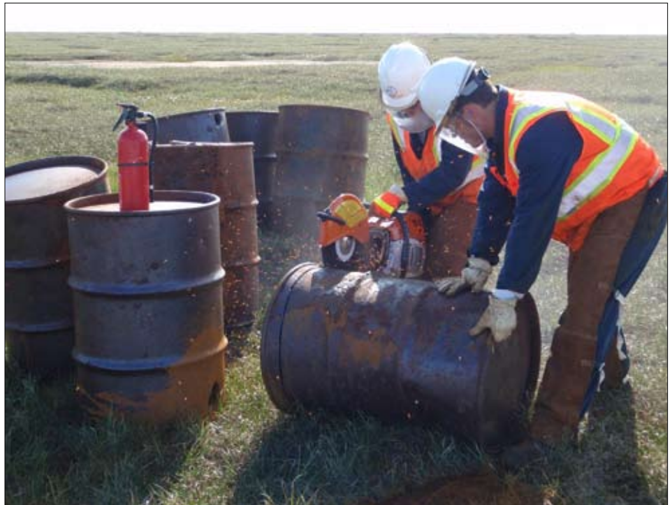
(Top photo) Darren Kayotuk (left) and Eric Jenks (right) use a demolition saw to dehead a drum before cleaning out residue inside. (Bottom photo) Eric Jenks (left), Mike Flisk (center), and Dave Vandergriff (right) process drums in Kaktovik. The drums are cleaned and crushed before being placed into a container for shipment to a metal recycler in Fairbanks. (Courtesy photos)
