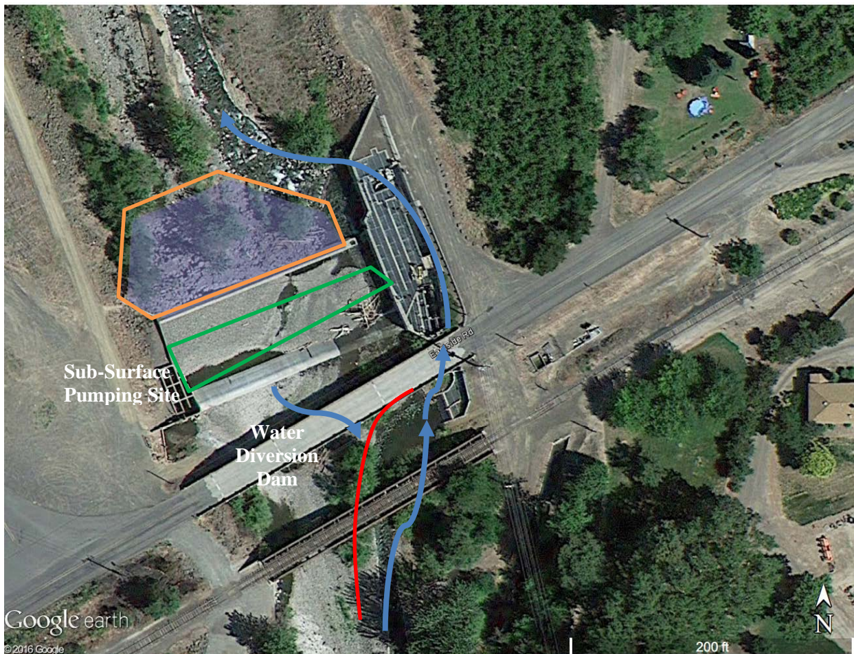
Figure 2-3: Aerial view of Nursery Bridge drop structure showing proposed diversion dams (red), pumping station (green), and work areas (orange) for the rip rap installation. Subsurface flows that find a way around the annual diversion dam are likely to enter the project site and may need to be diverted through pumping (blue).
