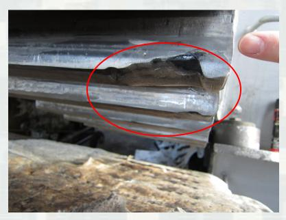
Damage to pinion gear teeth  Damage to ring gear teeth
