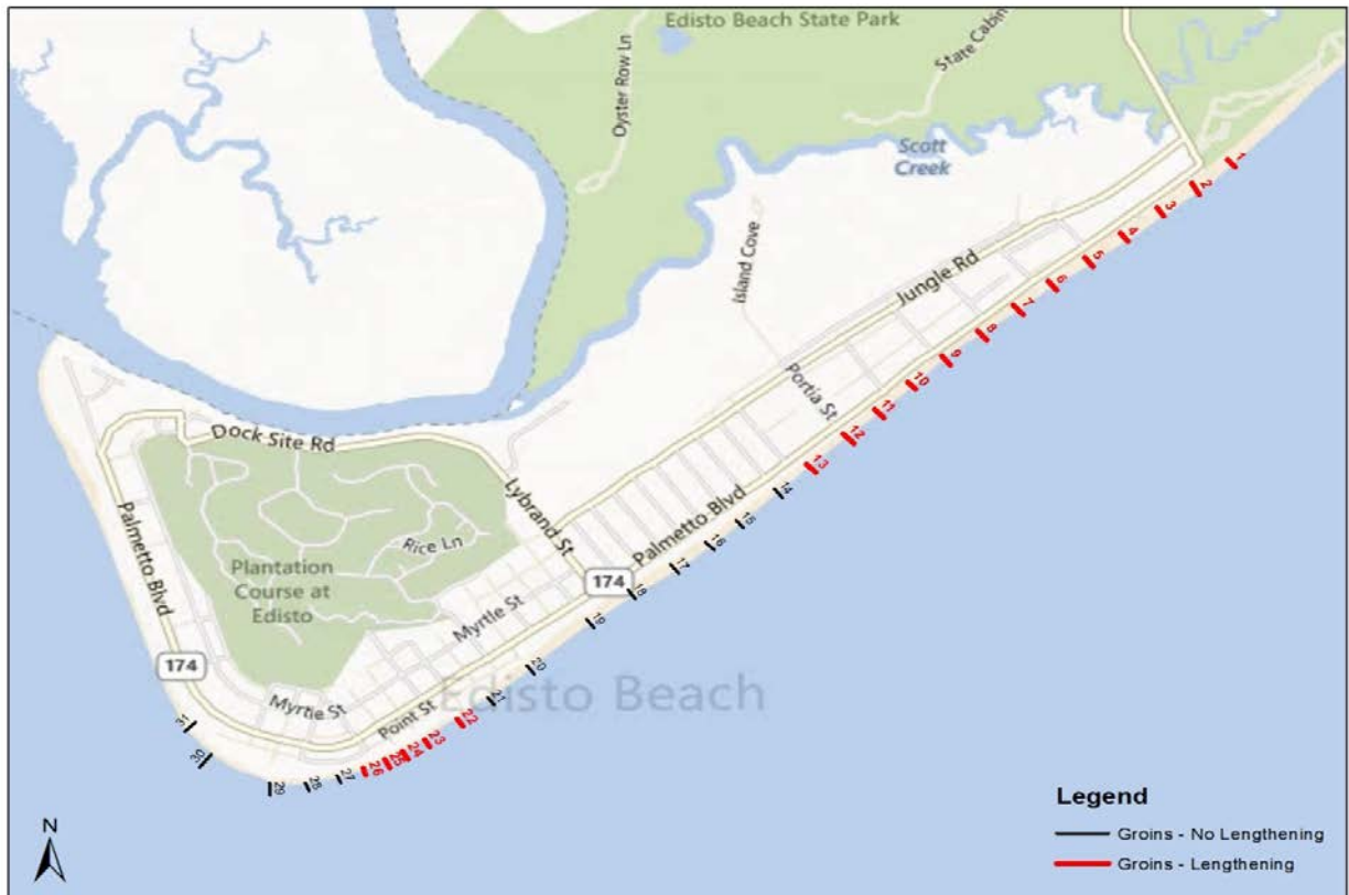
Figure 1.4-3 Existing groins to be lengthened
