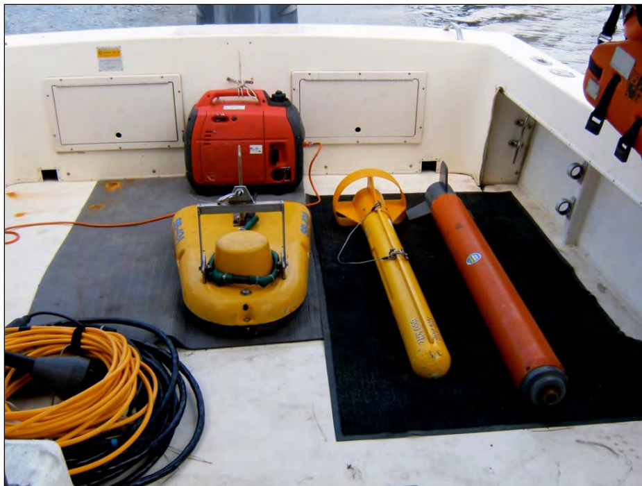
Figure 26. Survey instruments employed during the investigation included (from right to left) the magnetometer, the sidescan sonar, and the subbottom profiler. Honda generator employed to power the instruments is in the background adjacent to the transom.
