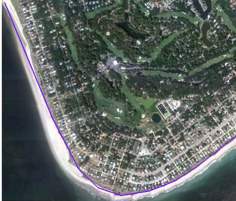
Figure 43: Without-project forecast of average shoreline position in 2064 along the inlet shoreline to Groin cell 21.
