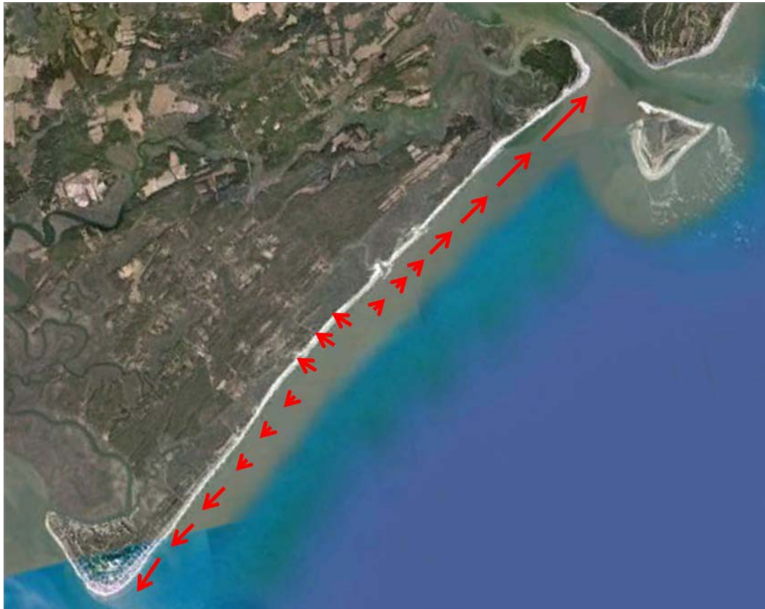
Figure 2: Longshore sand transport regime between North Edisto Inlet and South Edisto Inlet.
