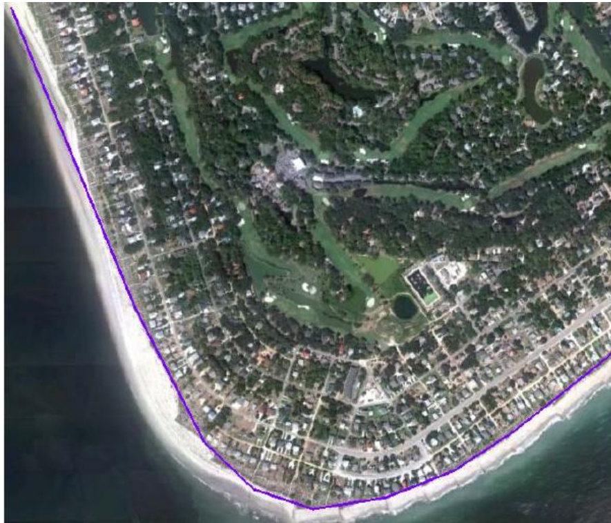
Figure 4.1: Predicted location of the shoreline between reaches I1 and E3 (purple line) after 50 years in the future without project scenario.
