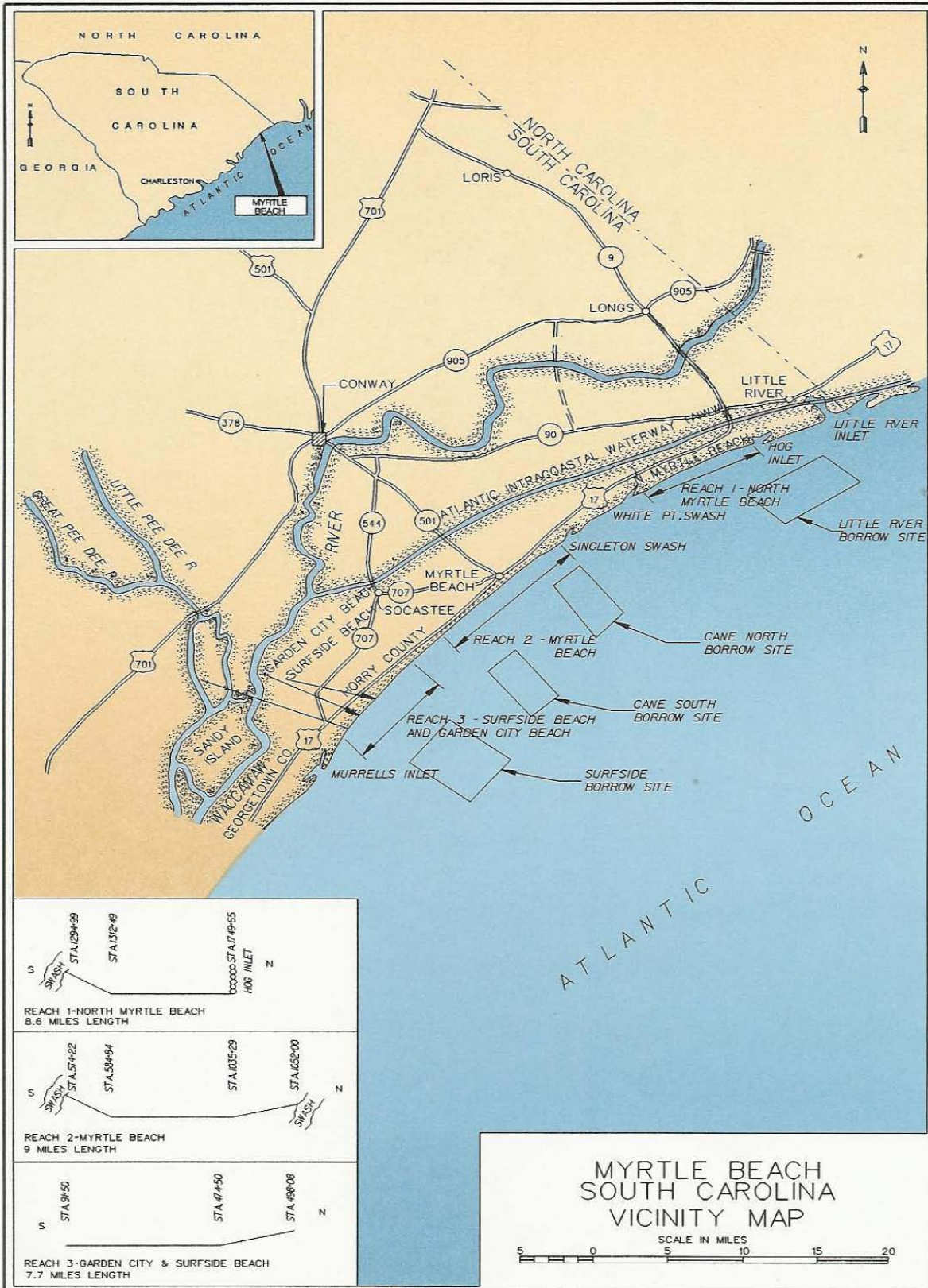
Figure 1: Offshore Borrow Areas
