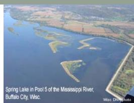
The project consisted of building islands along the west side of the lake and within the lake to restore habitat and diversity. Material was dredged from Spring Lake for island fill and topsoil to create additional deeper areas for fish habitat. The project will slow the degradation of about 200 acres of valuable backwater fish and wildlife habitat, directly affecting two-thirds of the lake.
