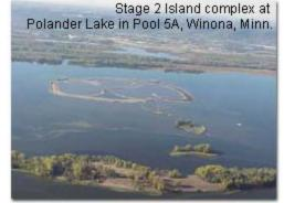
Stage 1 of the project included constructing a closure across a side channel carrying Pap Slough flows into the lake, a 1,000-foot rockfill island in the upper portion of the lake to reduce wave action and bank stabilization of two existing barrier islands. Stage 2 consisted of a 6,000-foot island complex in the lower portion of the lake to increase aquatic plant growth and dredging to provide deepwater fish habitat.
