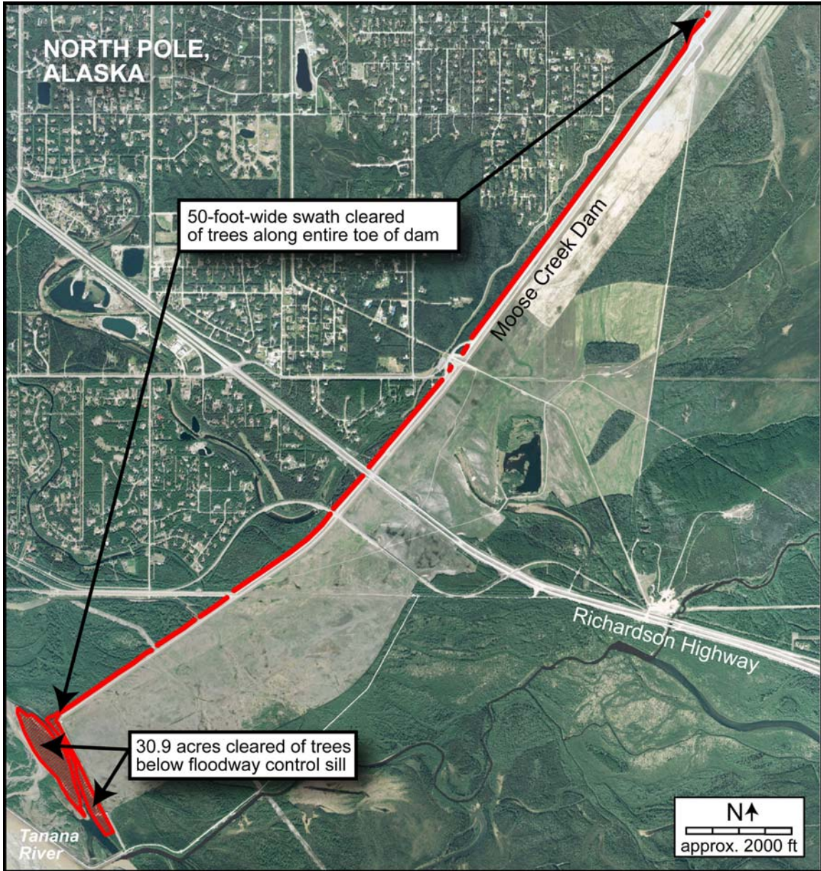
Figure 6. Southern segment of vegetation clearing at Moose Creek Dam and at the control sill.
