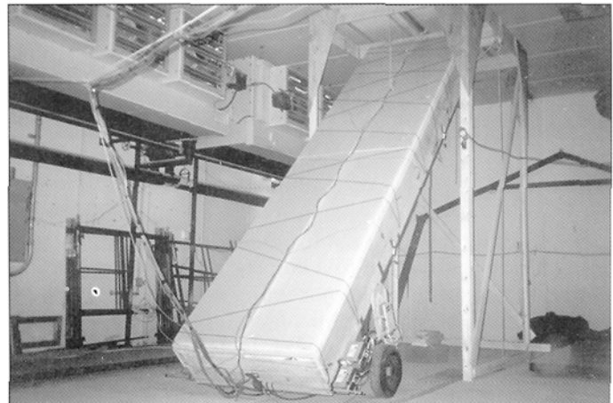
Figure 6. Test roof raised to 44 degree slope in the coldroom.
