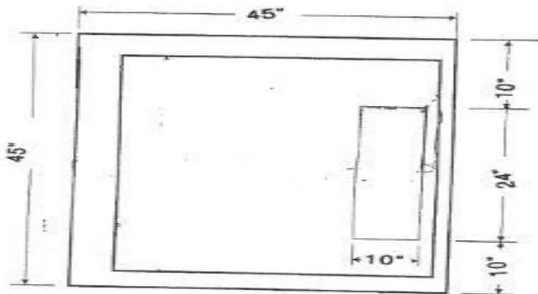
Note: Contractor to install all service entrance conduit in Secondary Side of pad opening.
