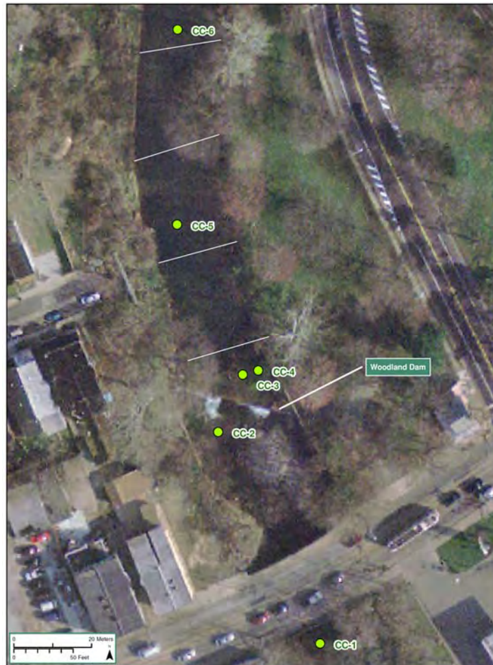
Figure 8. Sediment sampling locations for contaminant analysis at Woodland Dam. Transect lines indicate the locations of the sediment depth measurements.
