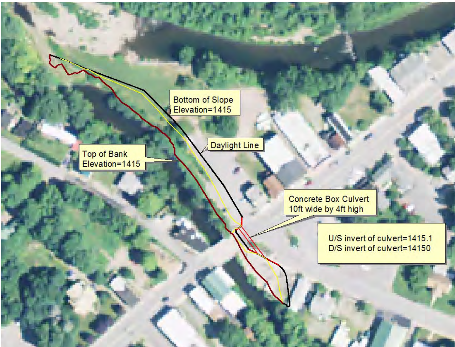
Figure 11.4 - Plan View of Post Interim Excavated Bench Downstream of Main Street Bridge
