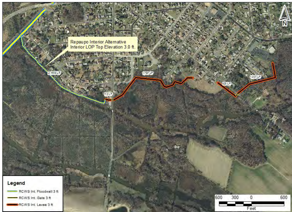
Figure 2-8: Repaupo 3ft NAVD Interior Levee Alternative
