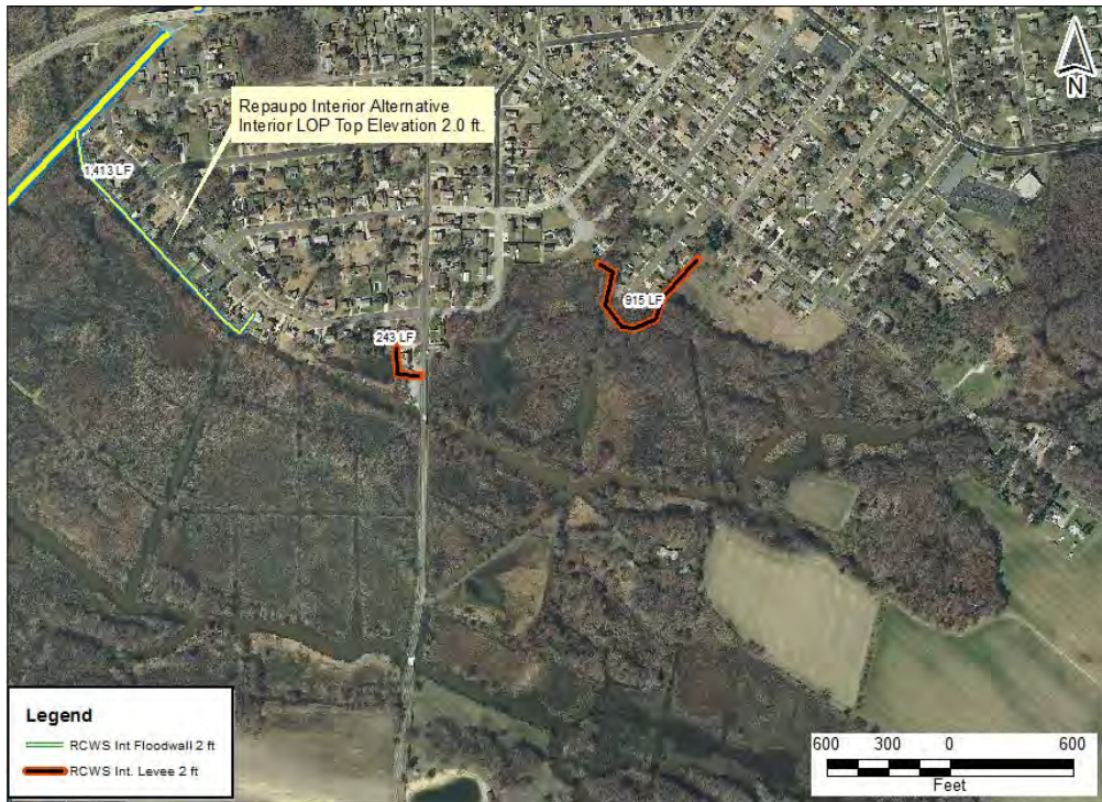
Figure 2-7: Repaupo 2ft NAVD Interior Levee Alternative
