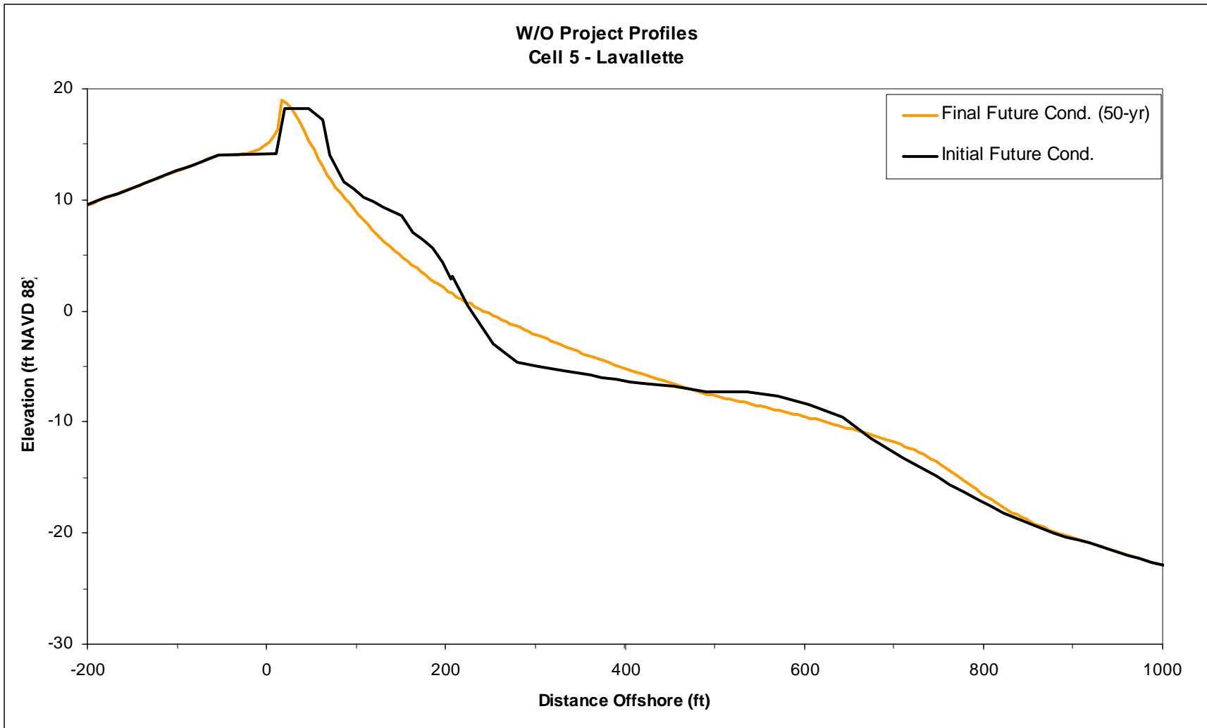
Figure 3-21 Pre- and Post 50-yr Storm Event Beach Profiles for Future Conditions for Cell 5 (Lavallette)
