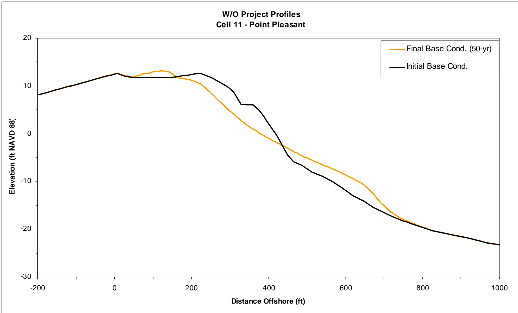
Figure 3-19 Pre- and Post 50-yr Storm Event Beach Profiles for Base Conditions for Cell 11 (Point Pleasant Beach)
