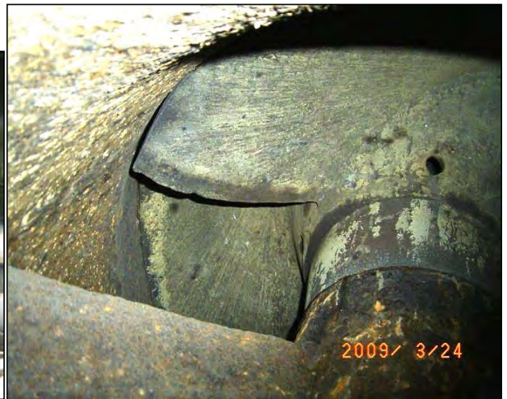
Nicked Impeller Blade
