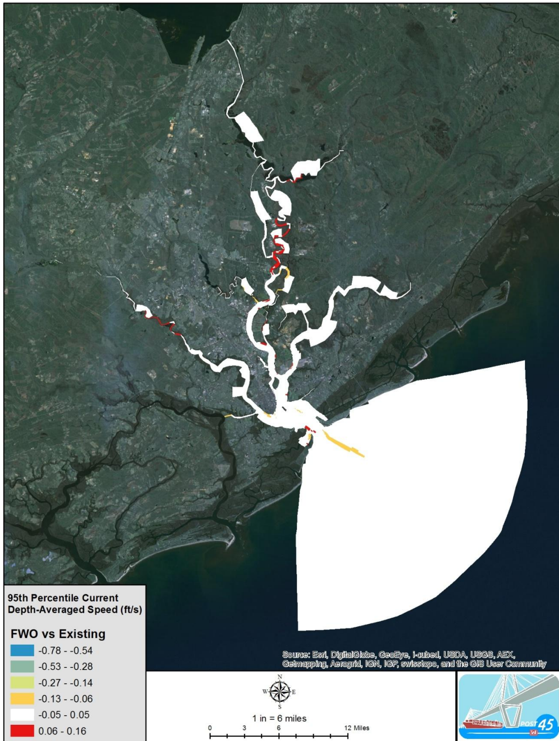
Figure 3.7.2 Future Without Change in 95 th percentile Depth-averaged Current Speed from Existing Condition
