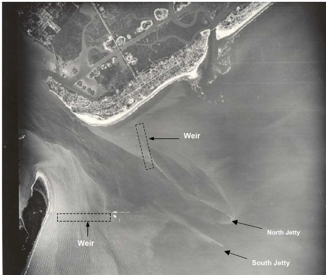
Figure 5.5.1 Charleston Harbor, 1968 showing weir-jetty structure and entrance channel.
