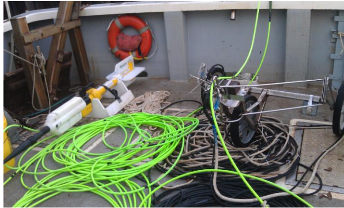
Figure 2. Top: Photograph of Klein 3000 dual frequency side scan sonar. Bottom: Geometrics G-882 marine magnetometer (left) and CCU's video tow system.
