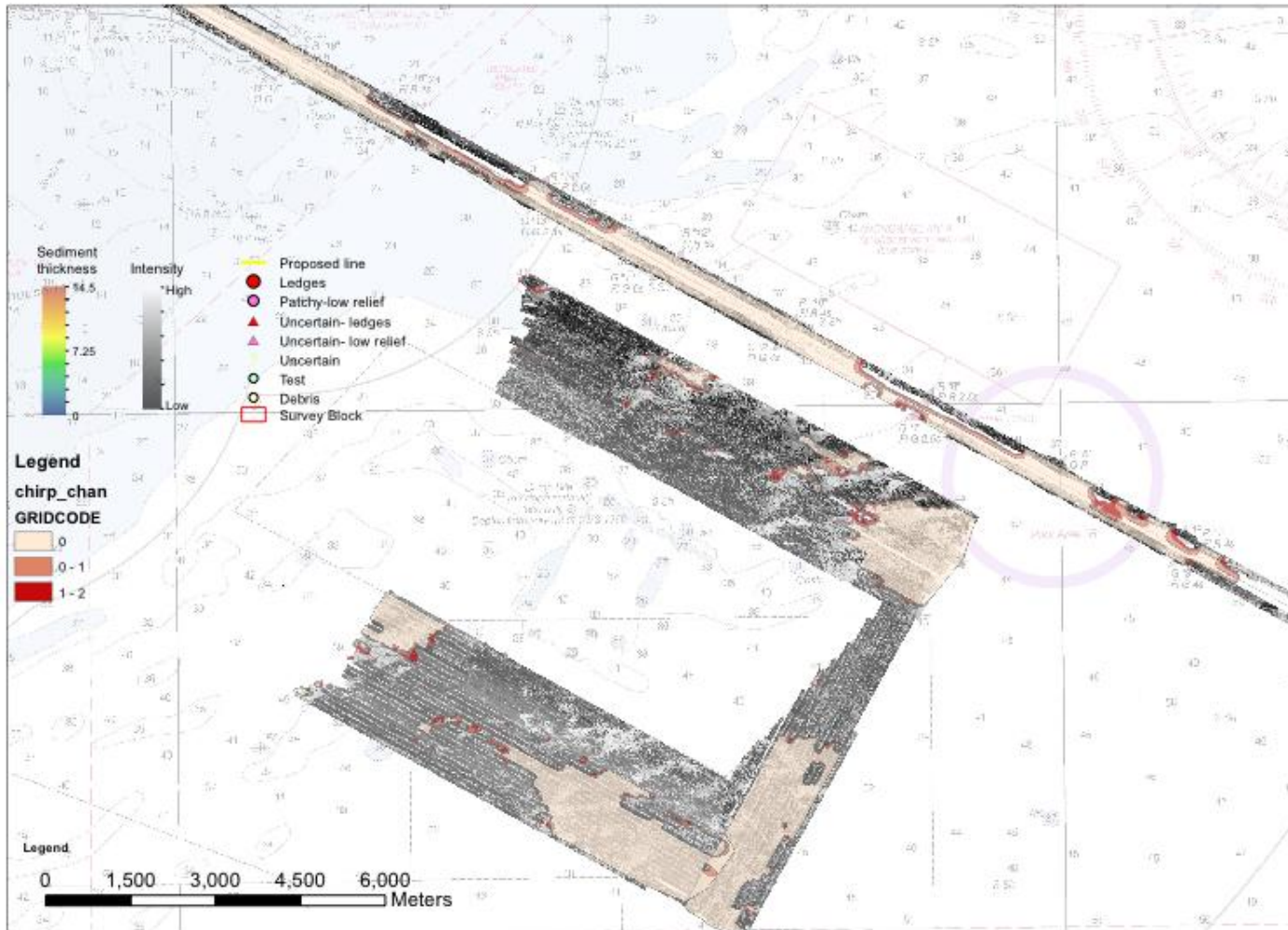
Figure 12. Side scan sonar (backscatter intensity) mosaic and Chirp (sediment thickness) in Post 45 ODMDS and entrance channel.
