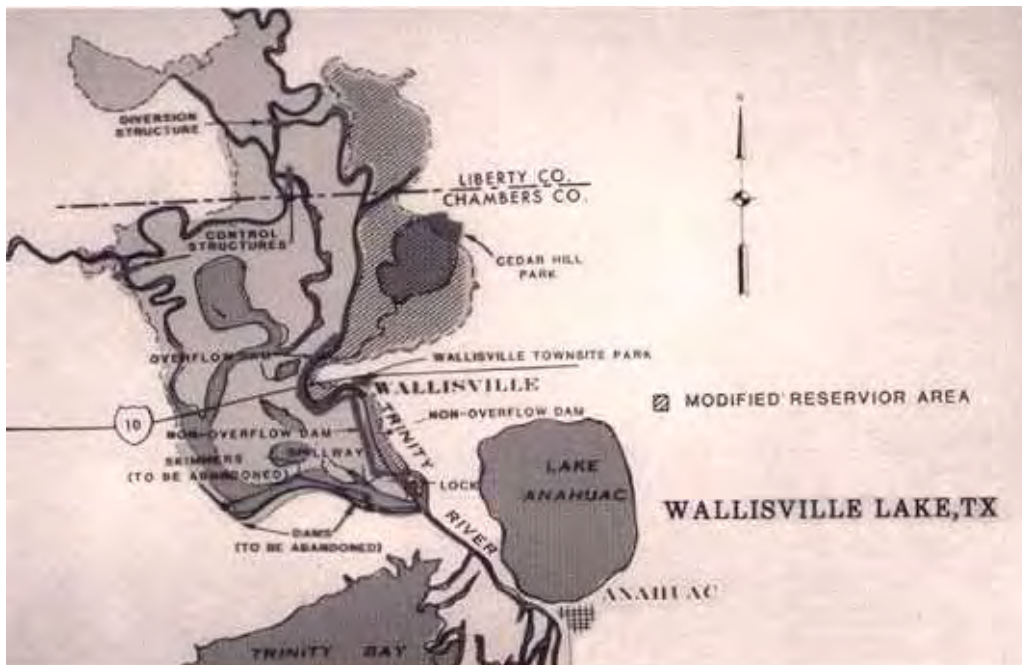
Left: Wallisville controversies and lawsuits illustrated the difficulty of reconciling engineering and environmental solutions. This map shows the redesign of Wallisville Lake.
