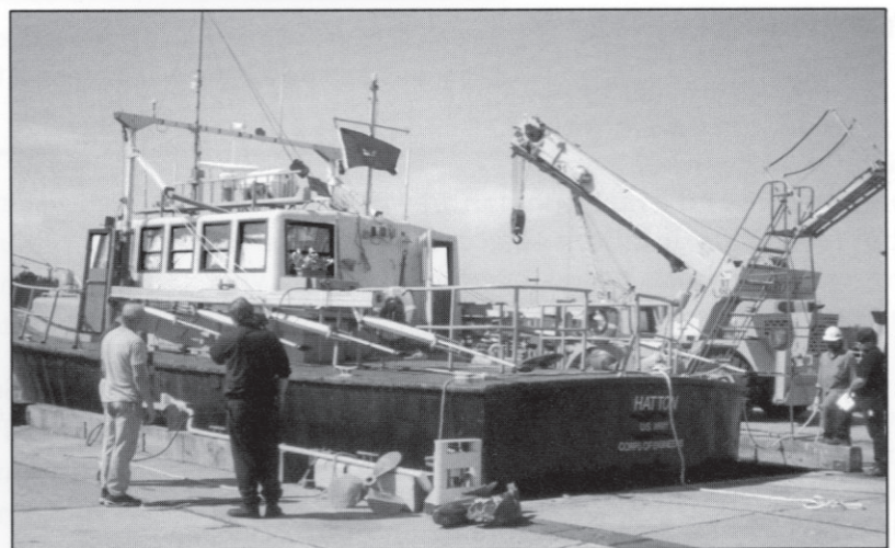
Extra time working during and following the world trade center attack required an early – albeit routine – maintenance call for the survey boat Hatton at Caven Point. Mechanics did the equivalent of a lube-oil-filter and adjusted the steering. The Hatton was back on the job in less than 24 hours.
