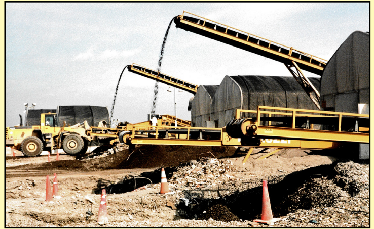
Debris moves between conveyor belts at the special landfill the Corps of Engineers managed on Staten Island for debris from the attacks. Unlike the Corps' more traditional debris missions, all of the debris from 9/11 had to be specially handled and examined for traces of evidence, human remains and/or personal affects. (Photo by Eric Reinert, USACE Office of History)
