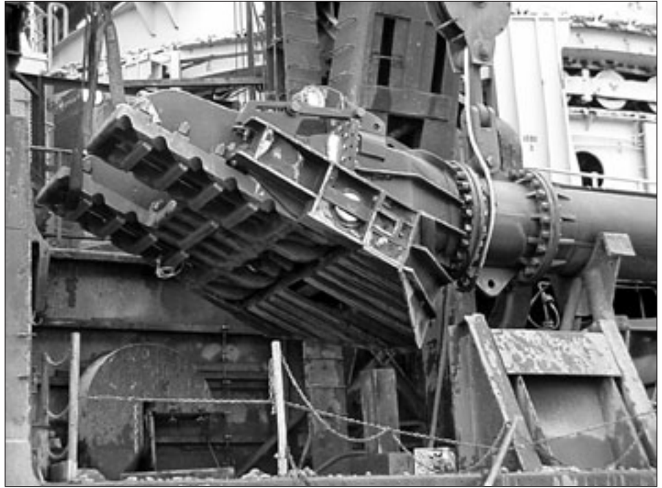
Turtle deflector visor designed by the Marine Design Center for the McFarland
