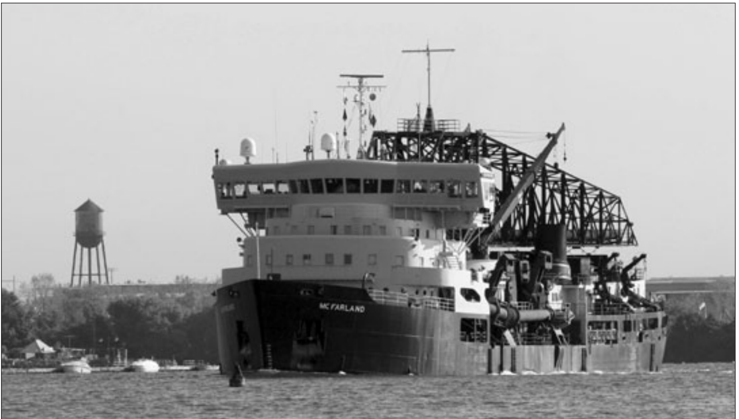
The Hopper Dredge McFarland, with unique triple capability for hopper, pipeline, and sidecast dredging
