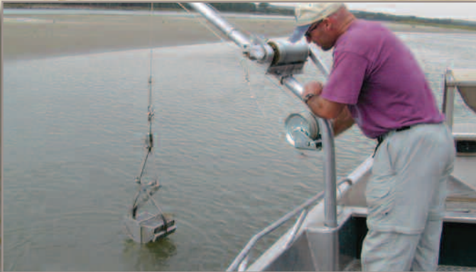
Using PONAR to grab samples of lake bottom material for analysis. The sampler is named after Great Lakes scientists, Charles E. Powers, Robert A. Ogle, Jr., Vincent E. Noble, John C. Ayers, and Andrew Robertson
