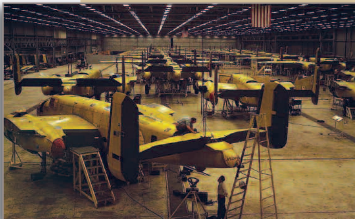
Assembling B-25 bombers at North American Aviation, Kansas City, KS, 1942 (Photo courtesy Library of Congress, LC-USW36-238)
