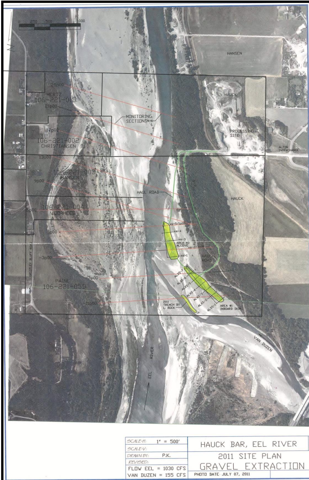
FIGURE E2: Example pre-extraction aerial photo w/ extraction zone cross sections delineated.
