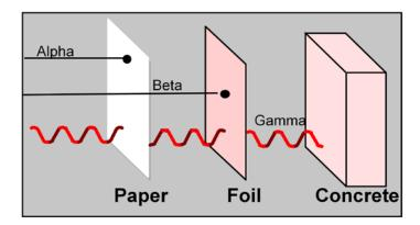
Radiation cannot be detected by human senses. For example it cannot be seen, heard, smelled, or tasted. However, it can be detected by instruments specificilly designed to measure the type and energy of radiation released during a radioactive decay. Examples of such detectors used at FUSRAP sites include geiger counters, scintillators, gamma spectroscopy detectors and personnel dosimeters.
