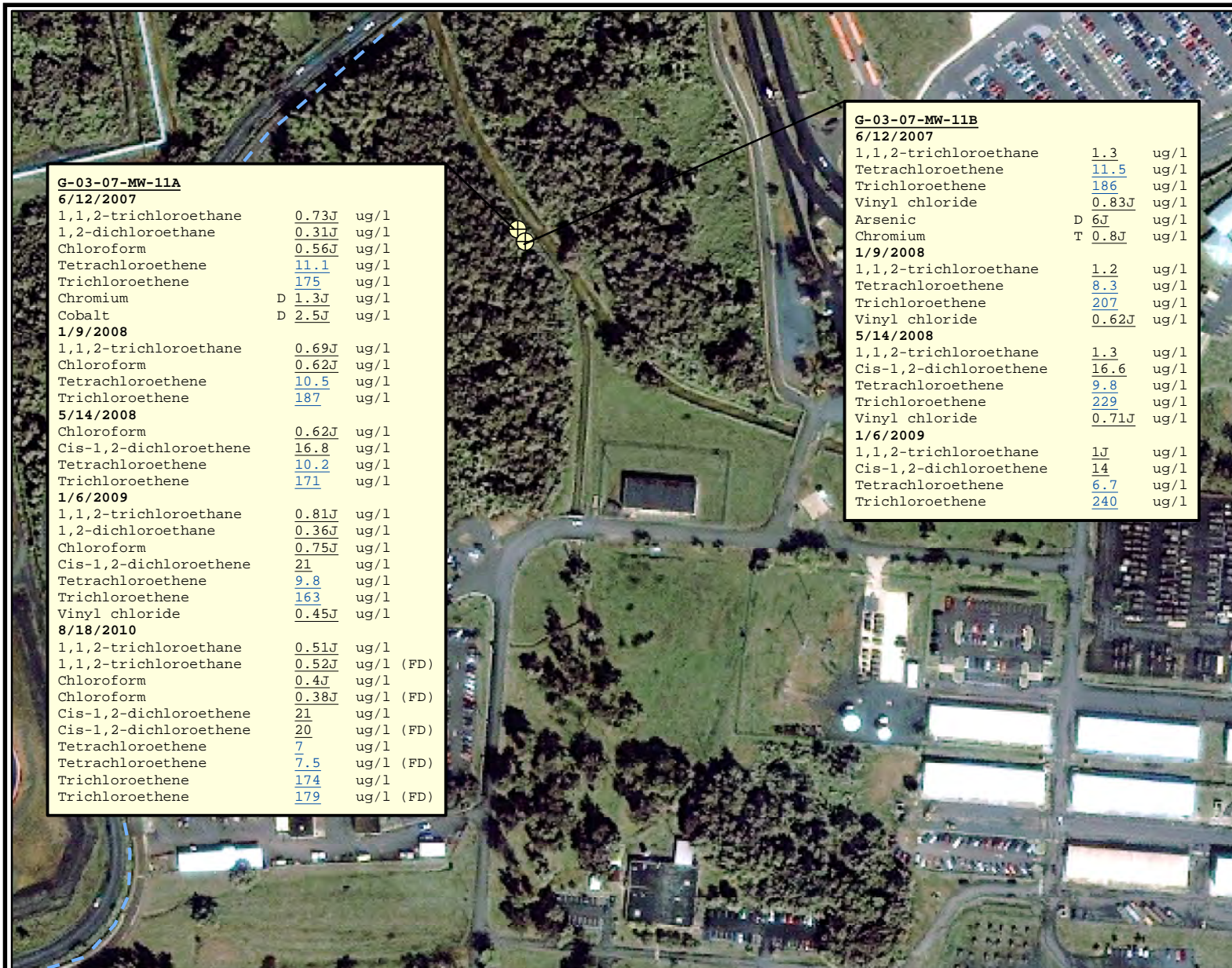
Figure 5-2 Groundwater Sample Locations and Concentrations Above Criteria at Site 1/SWMU 1
