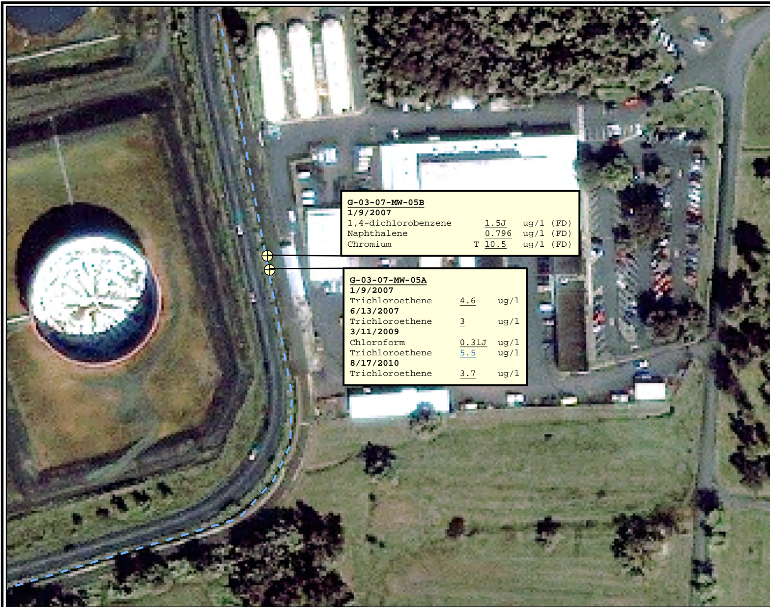
Figure 5-6 Groundwater Sample Locations and Concentrations Above Criteria at Site 3/SWMU 4
