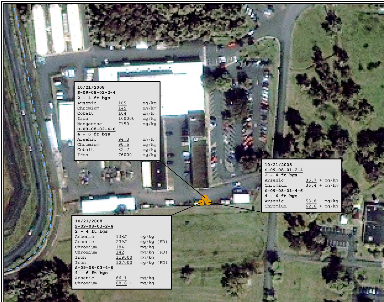
Figure 5-13 Soil Sample Locations and Concentrations Above Criteria at Site 9
