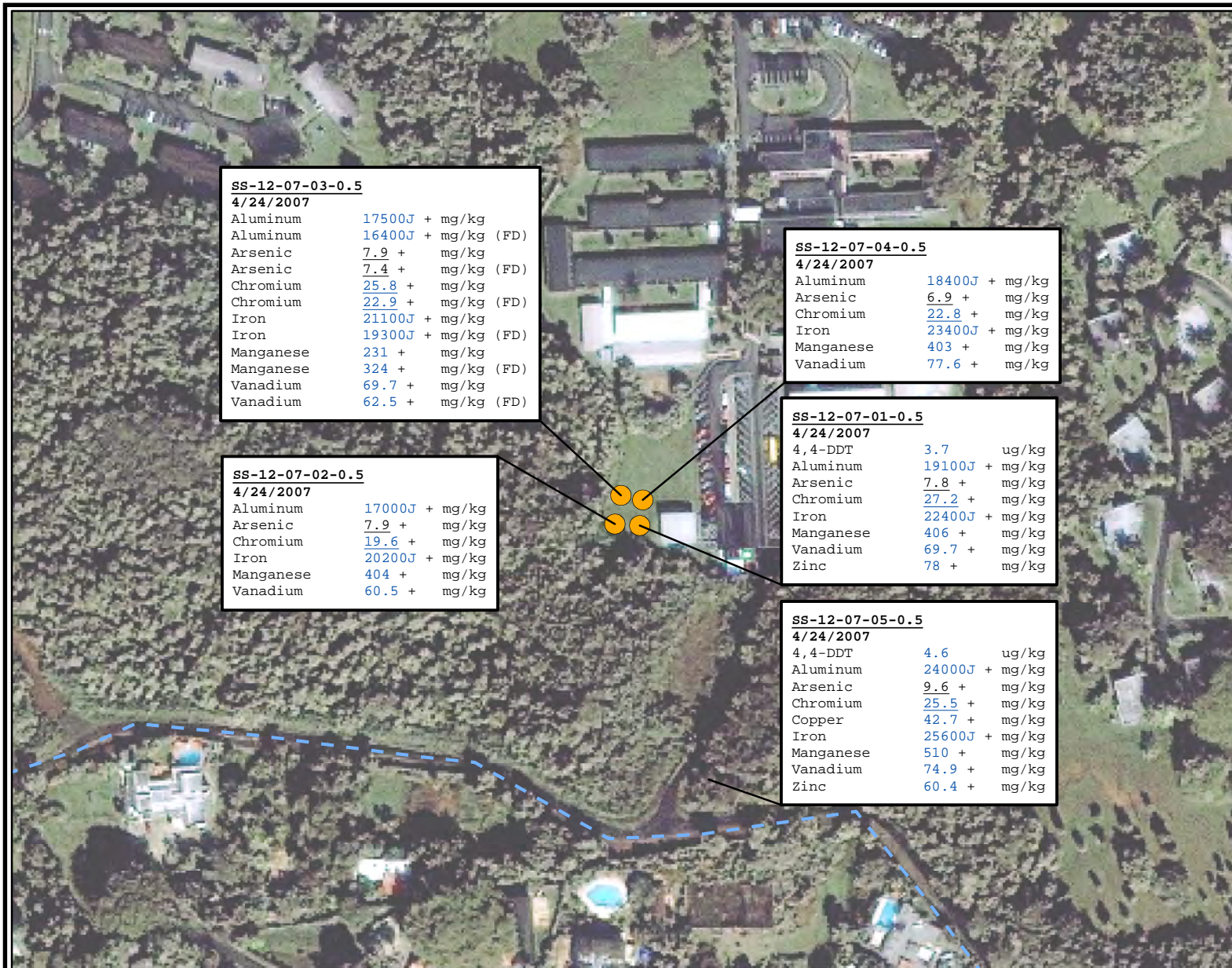
Figure 5-16 Soil Sample Locations and Concentrations Above Criteria at Site 12
