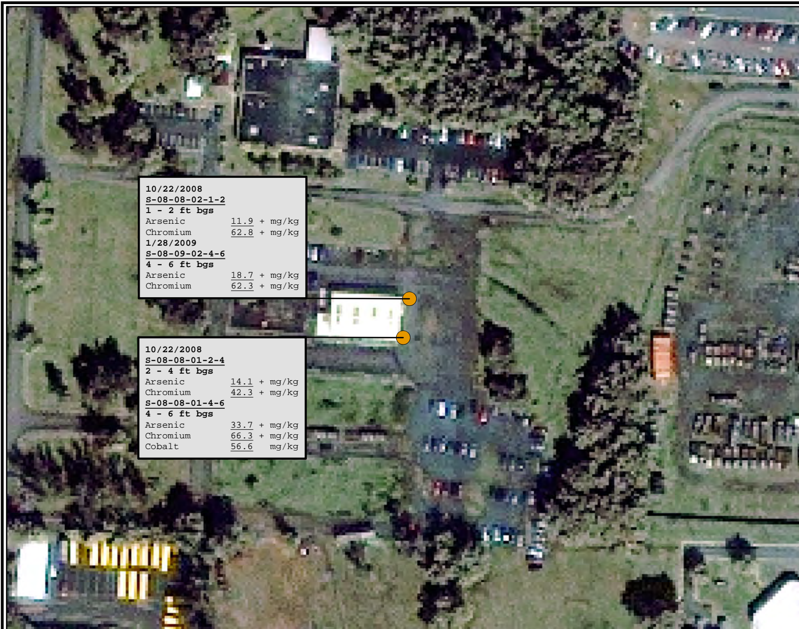
Figure 5-11 Soil Sample Locations and Concentrations Above Criteria at Site 8
