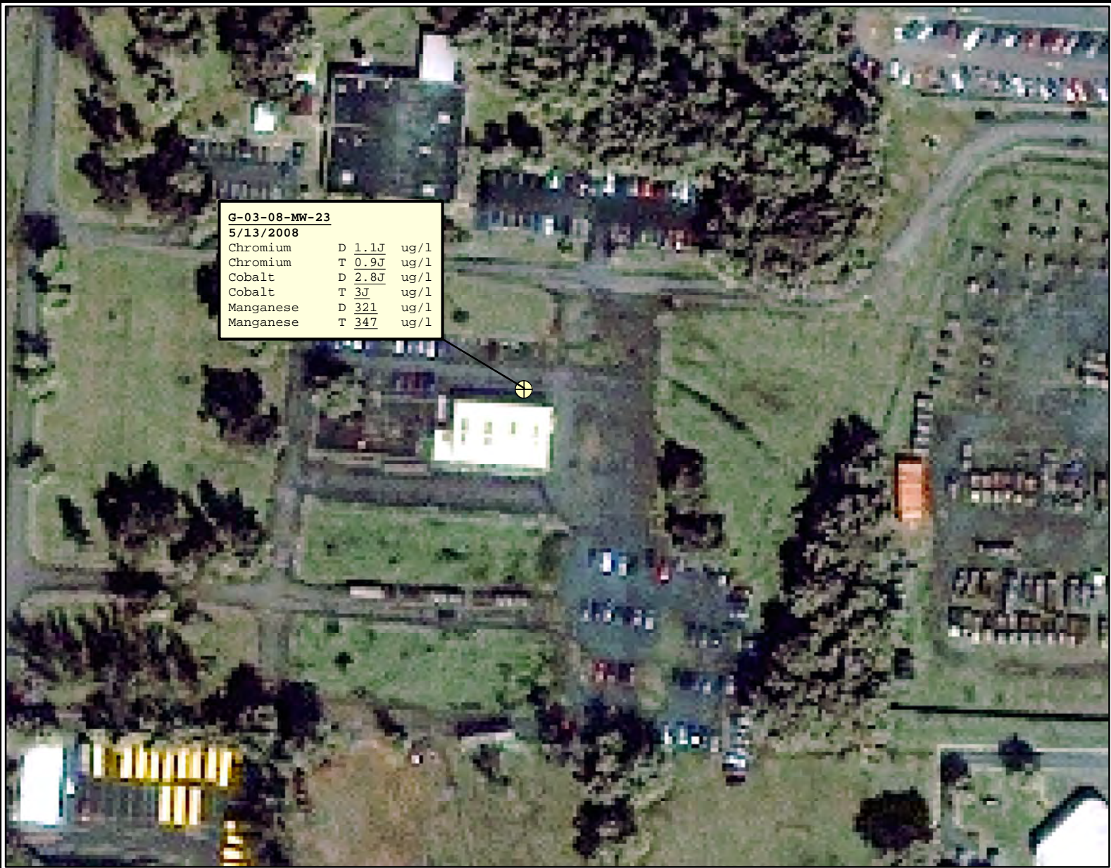
Figure 5-12 Groundwater Sample Locations and Concentrations Above Criteria at Site 8
