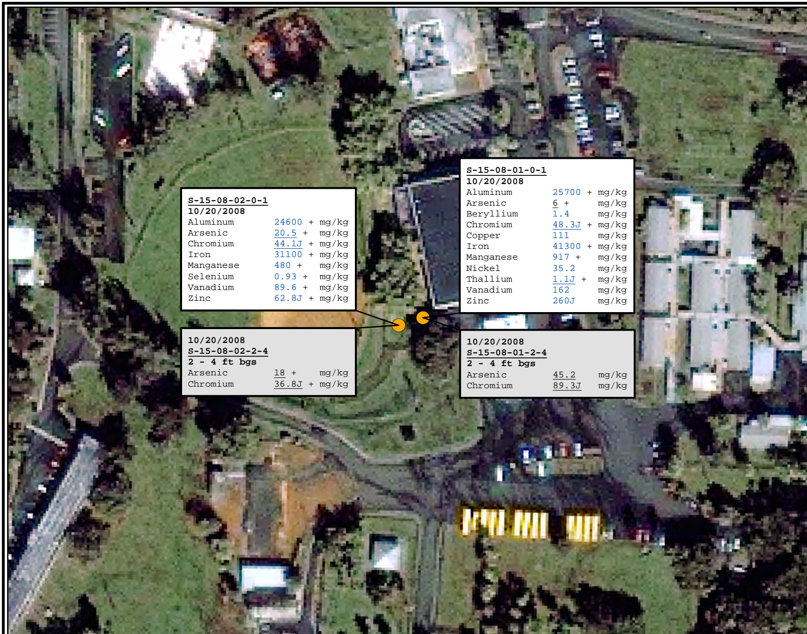
Figure 5-20 Soil Sample Locations and Concentrations Above Criteria at Site 15
