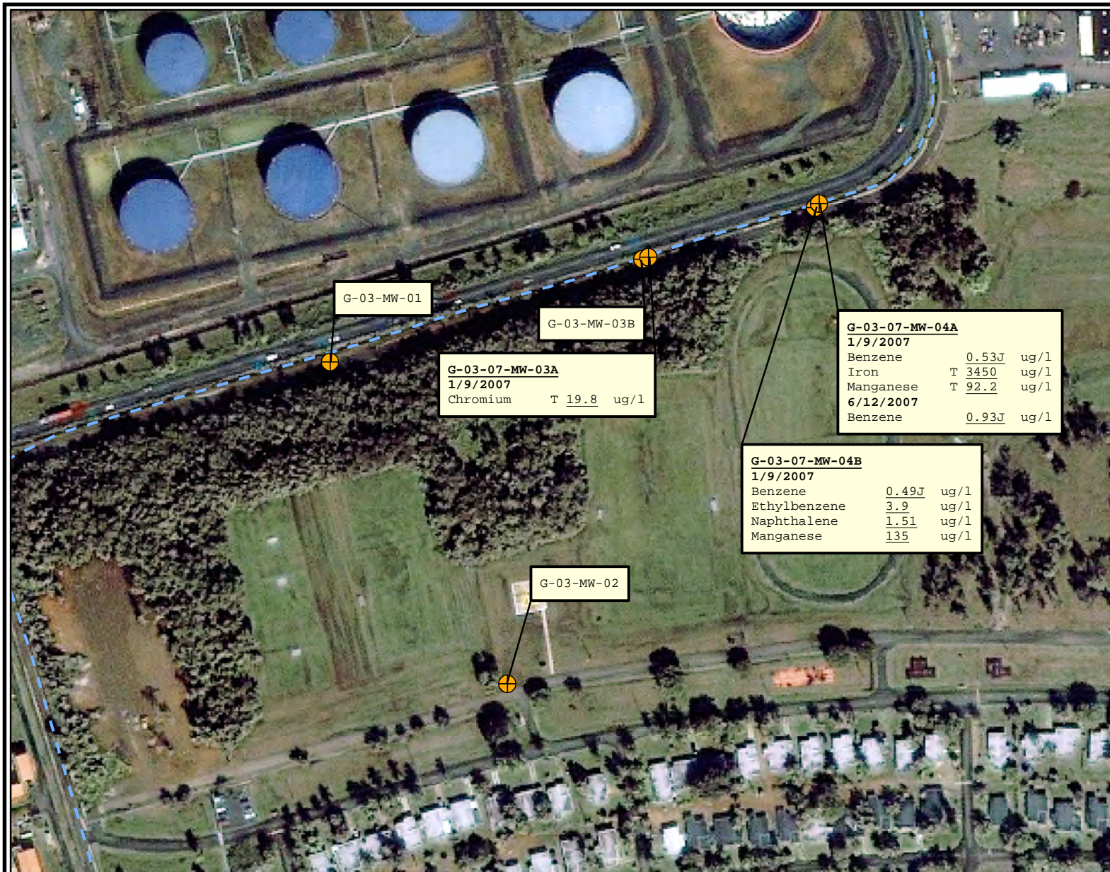
Figure 5-4 Groundwater Sample Locations and Concentrations Above Criteria at Site 2/SWMU 3
