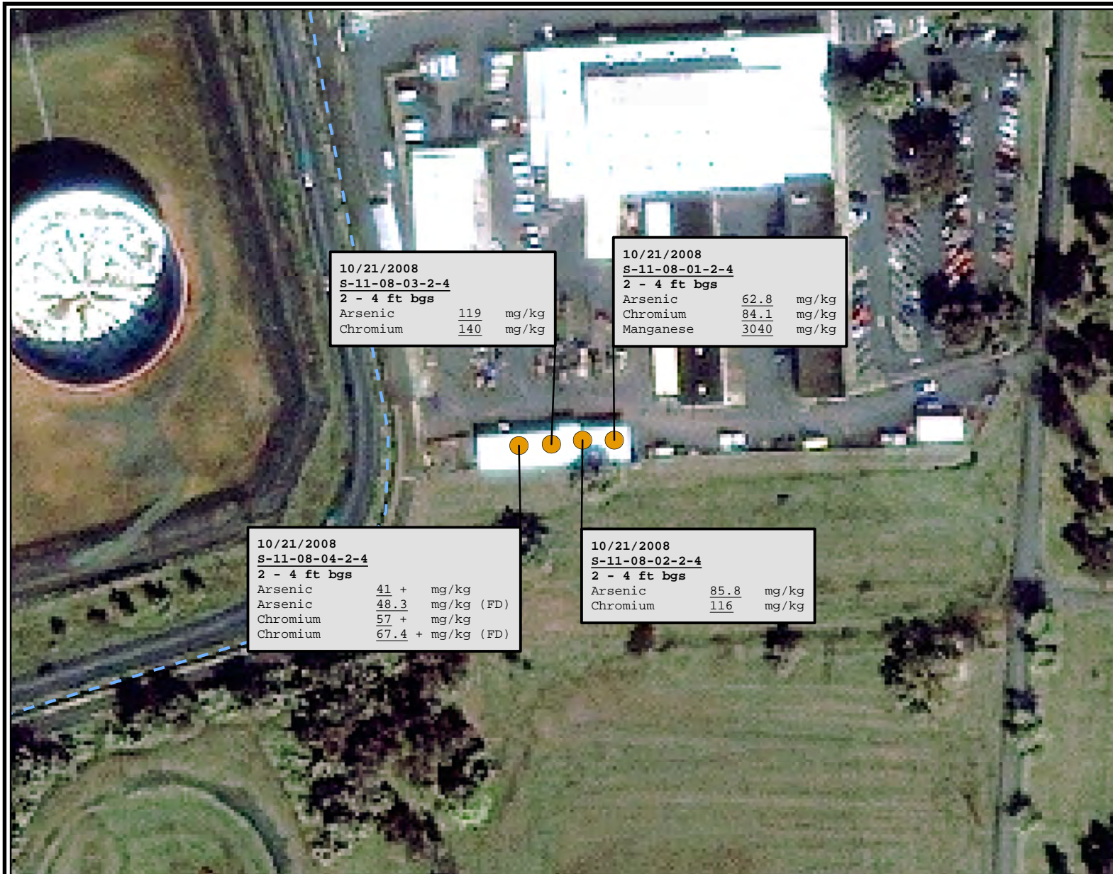
Figure 5-15 Soil Sample Locations and Concentrations Above Criteria at Site 11
