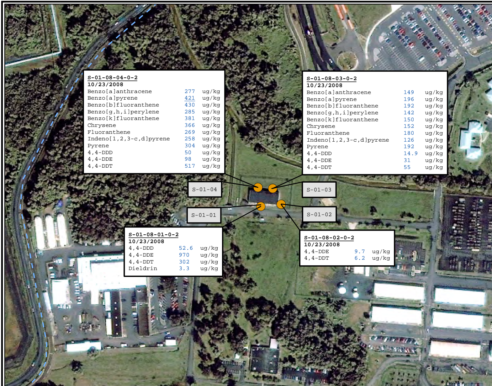
Figure 5-1 Soil Sample Locations and Concentrations Above Criteria at Site 1/SWMU 1
