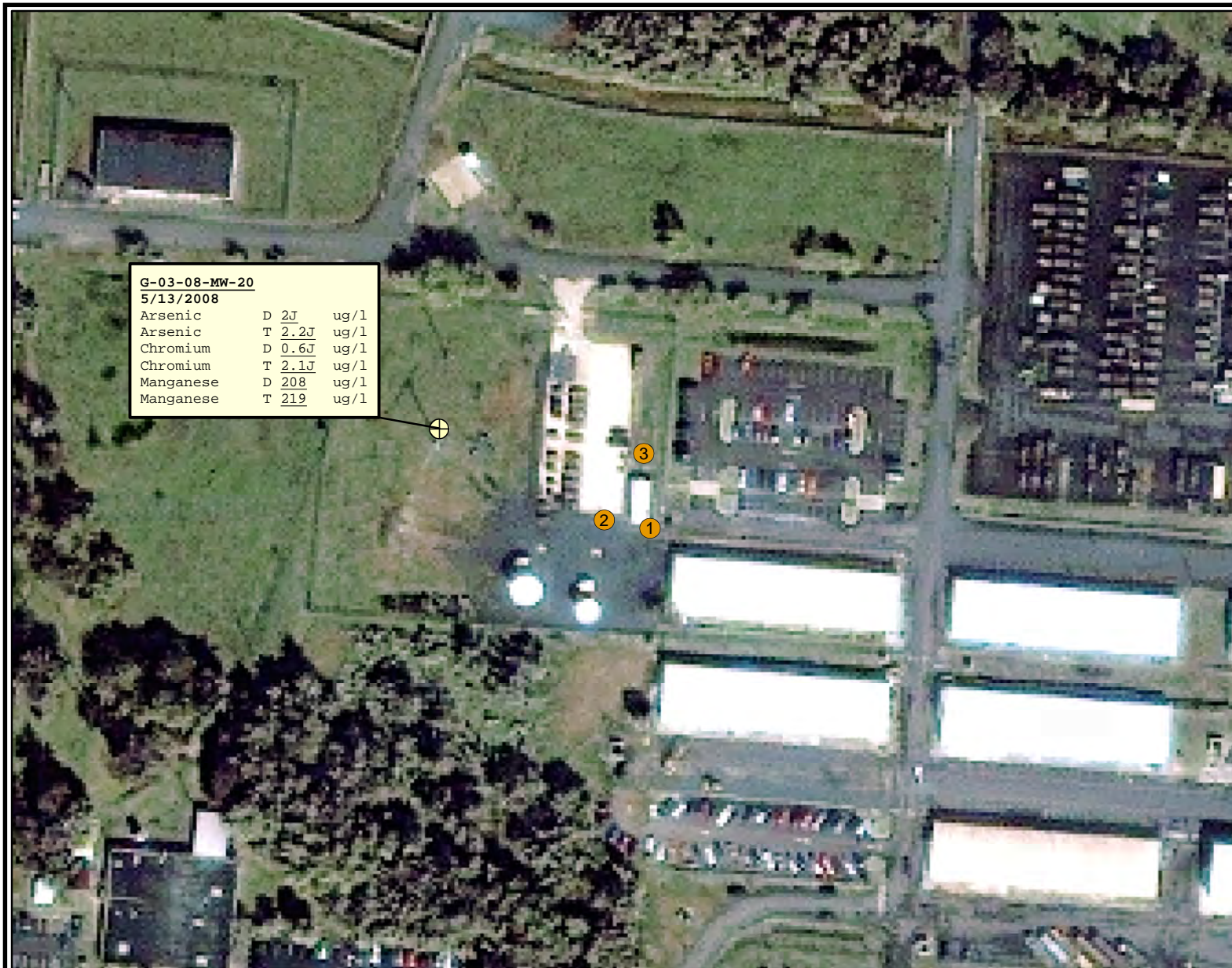
Figure 5-14 Groundwater and Soil Sample Locations and Concentrations Above Criteria at Site 10
