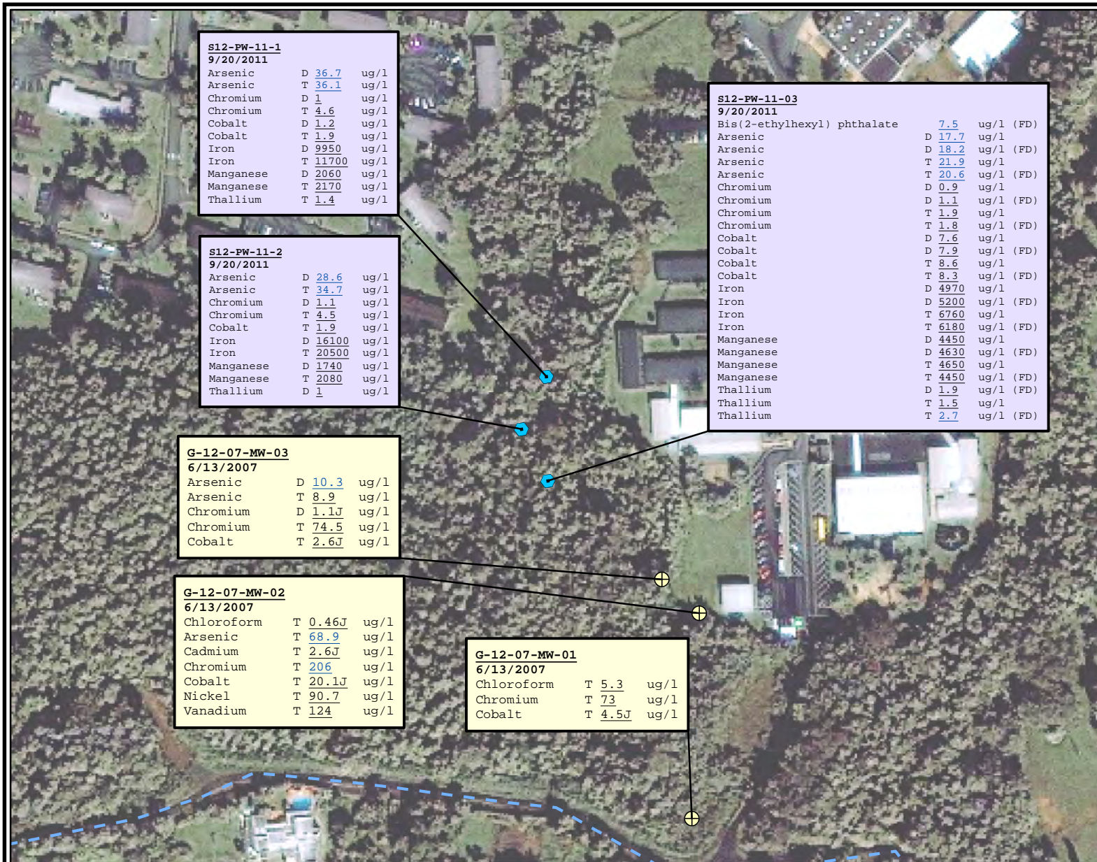
Figure 5-18 Pore Water and Groundwater Sample Locations and Concentrations Above Criteria at Site 12
