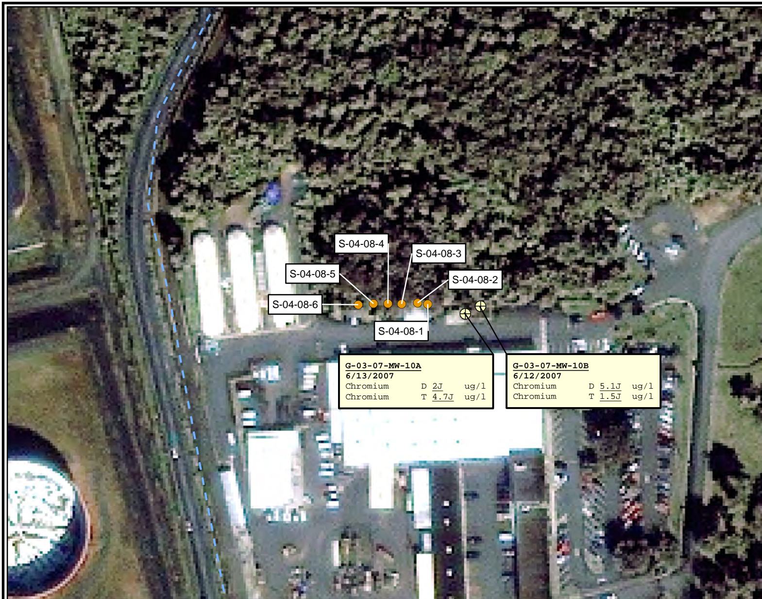
Figure 5-7 Groundwater and Soil Sample Locations and Concentrations Above Criteria at Site 4/SWMU 5
