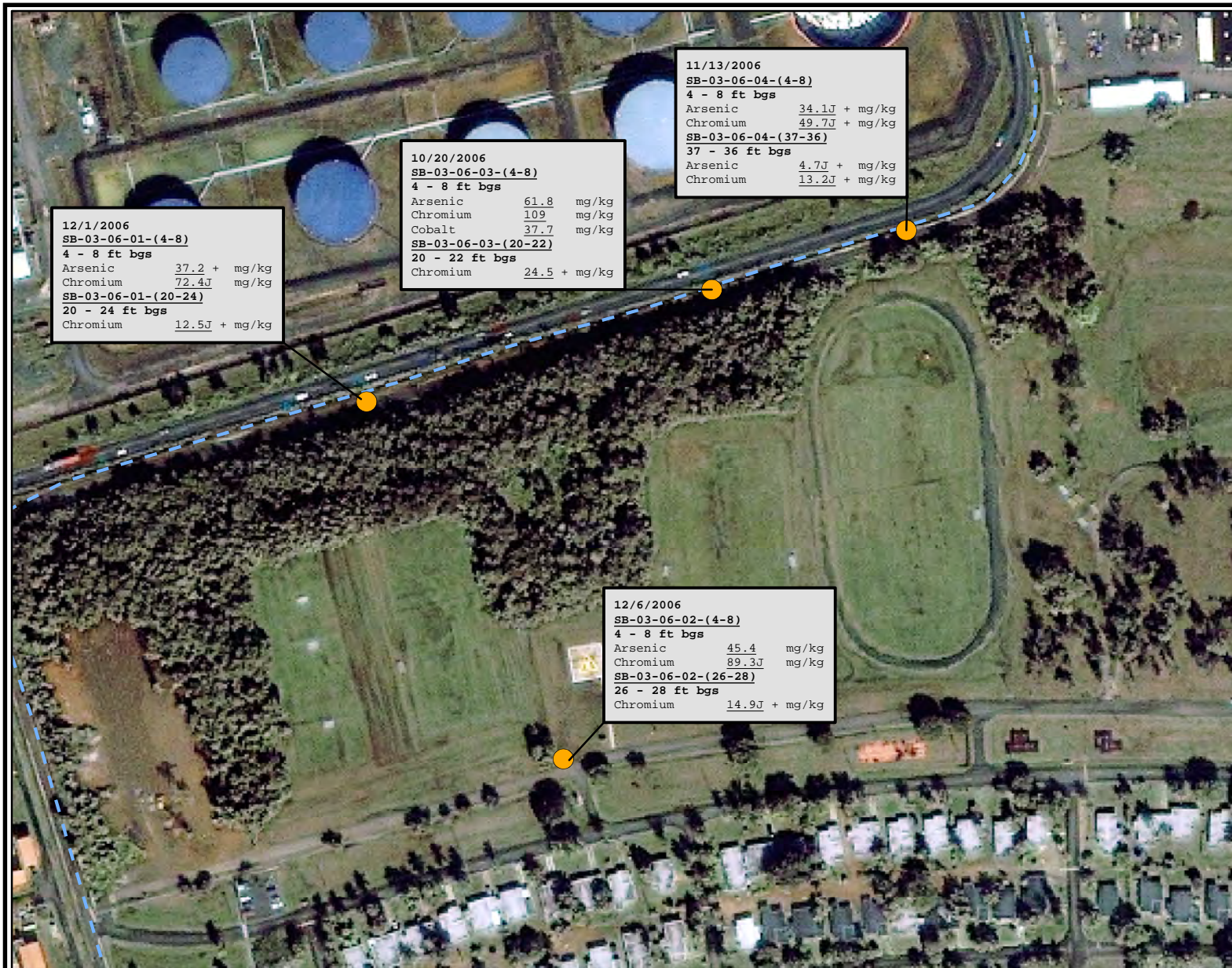
Figure 5-3 Soil Sample Locations and Concentrations Above Criteria at Site 2/SWMU 3
