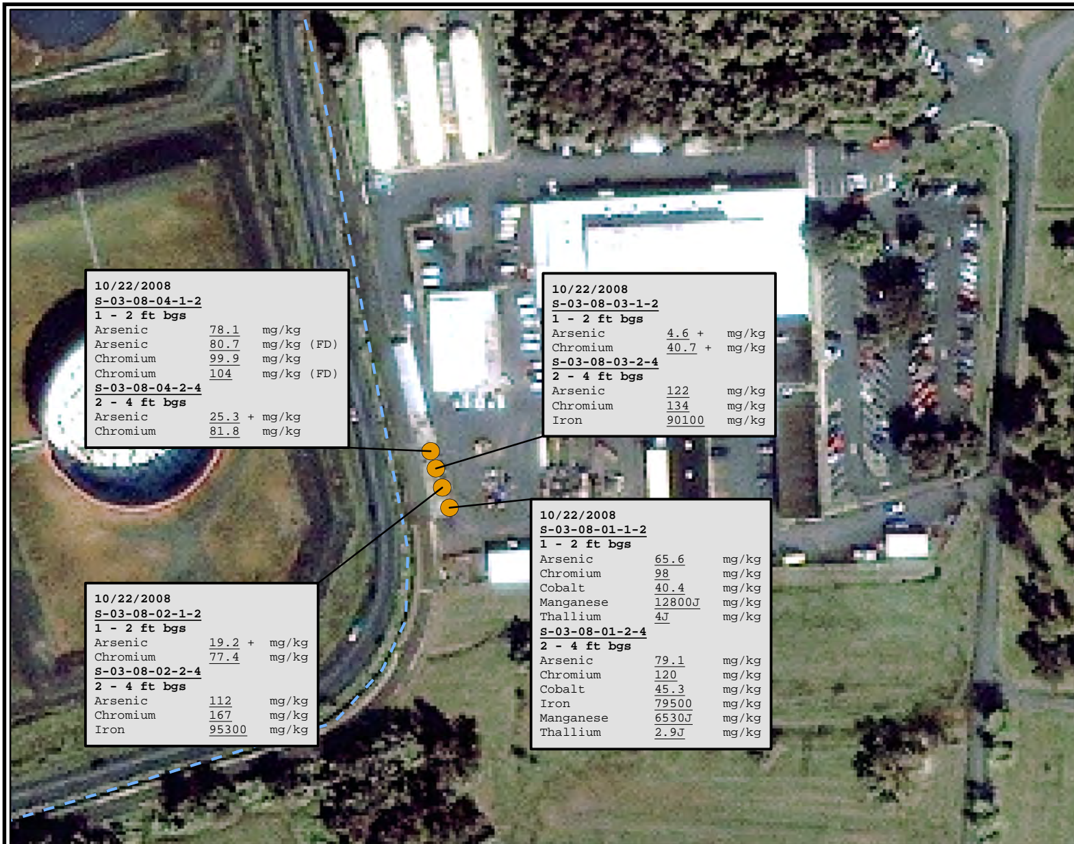
Figure 5-5 Soil Sample Locations and Concentrations Above Criteria at Site 3/SWMU 4
