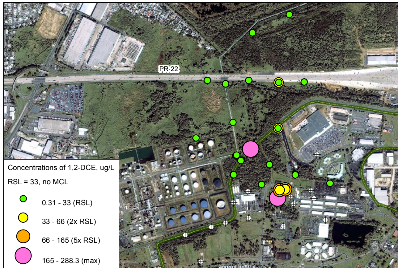
Relative Concentrations of Tetrachloroethene and Its Degradation Products
