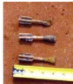
Tail assemblies belonging to the M-101 spotting round (above) found by contractors clearing the impact area at Schofield Barracks.
