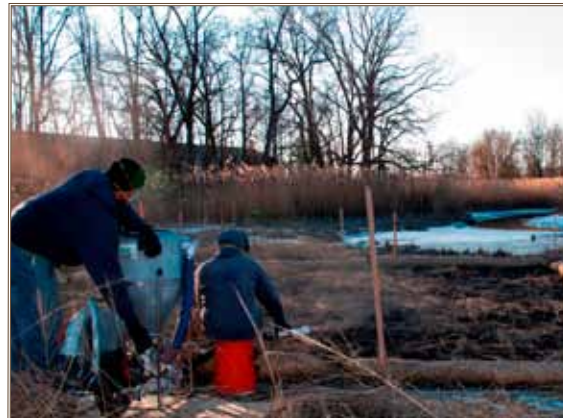
Activated carbon pellets are applied to an upper creek wetland at APG as part of a study utilizing activated carbon as a means of sequestering or isolating harmful contaminants from being stored in the organs or body tissues of aquatic organisms and animals. Photo courtesy APG Public Affairs Office.
