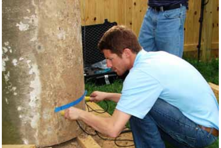
Alec Liebman performs ultrasonic testing on a historic gate component at Arlington National Cemetery. The testing measures the stone's consistency and condition, helping to determine conservation needs. The gates are being evaluated by historic preservation experts who catalog the components and assess their condition. Arlington officials plan to restore these gates and incorporate them into future expansion projects in the cemetery. (U.S. Army Corps of Engineers photo by Lauren McCroskey)
