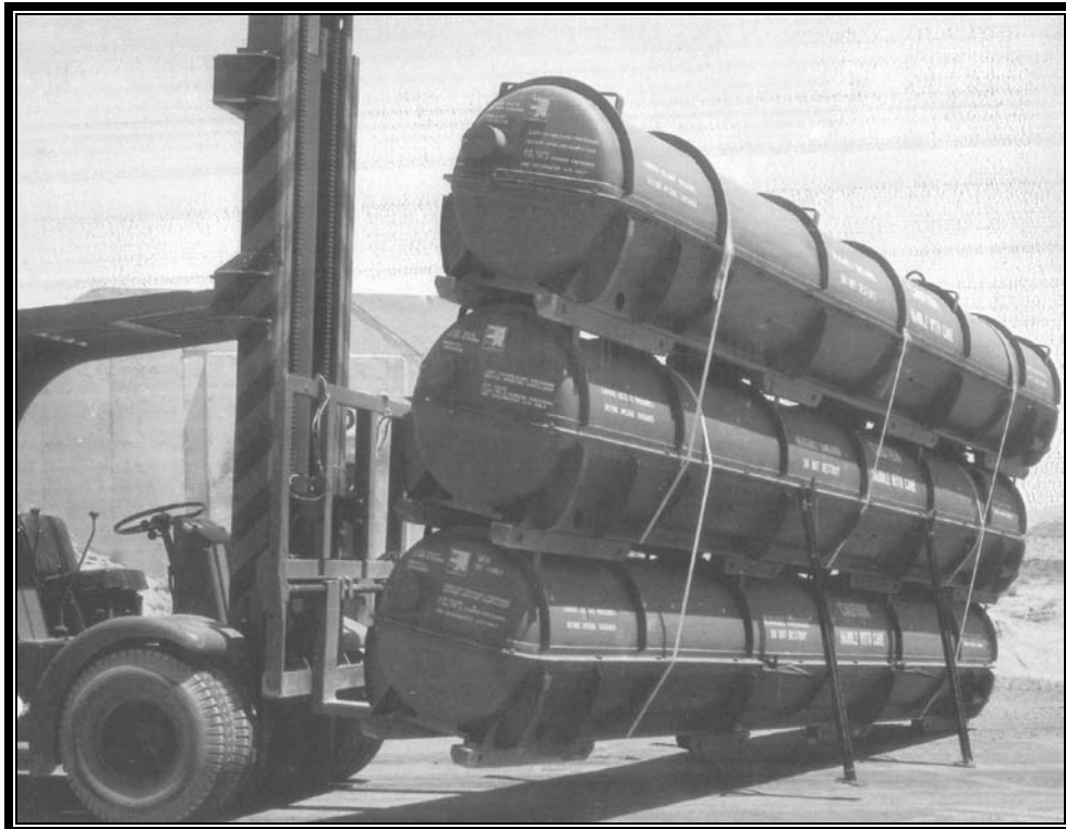
Plate 7.5 Bundle of three NIKE missiles. Note steel cables on forklift frame and stabilizers attached to center missile container (Sierra Ordnance Depot 1955:n.p.)
