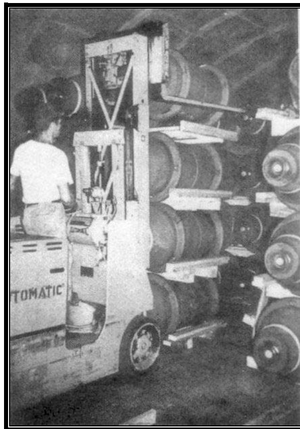
Plate 6.21 “Bomb being placed on fourth tier on wooden dunnage” (Facilities Section 1950:n.p.)
