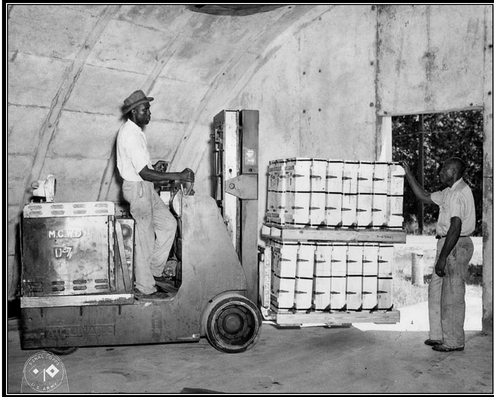
Plate 6.18 Handling palletized ammunition with electric forklift, ca. 1950 (Courtesy U.S. Army)
