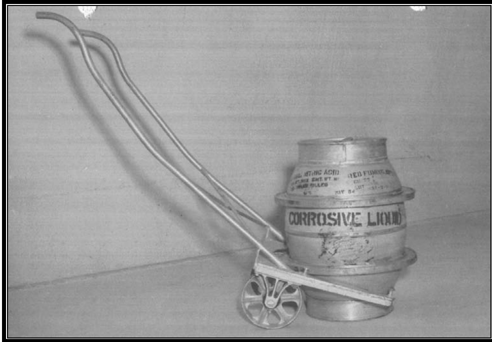
Plate 7.6 Container of inhibited red fuming nitric acid and specially designed handling cart (Sierra Ordnance Depot 1955:n.p.)
