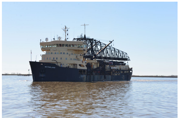
Feb. 16 - The Hopper Dredge McFarland works to keep the deep draft channel open in the lower Mississippi River. (Photo by the USACE, New Orleans District)
