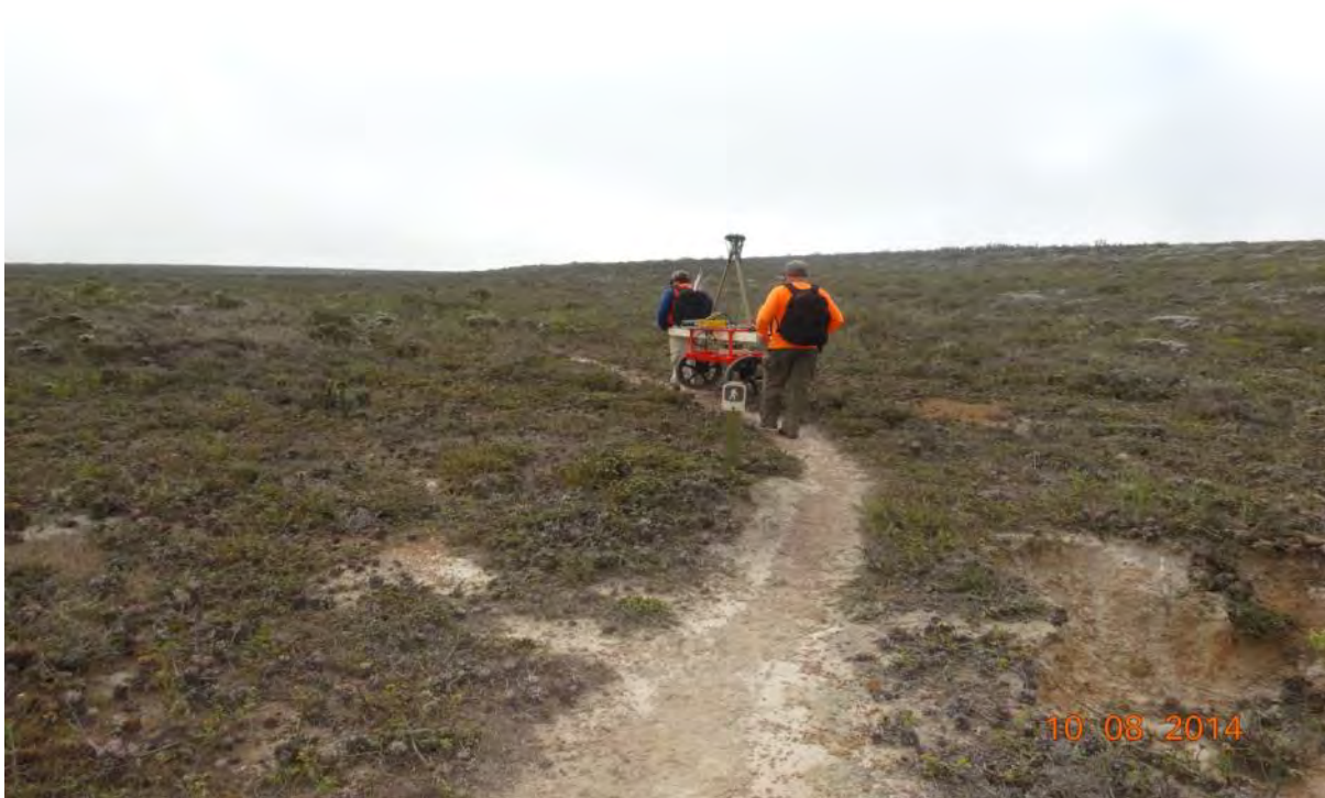
Photograph 19 EM61 carrying unit along trail
