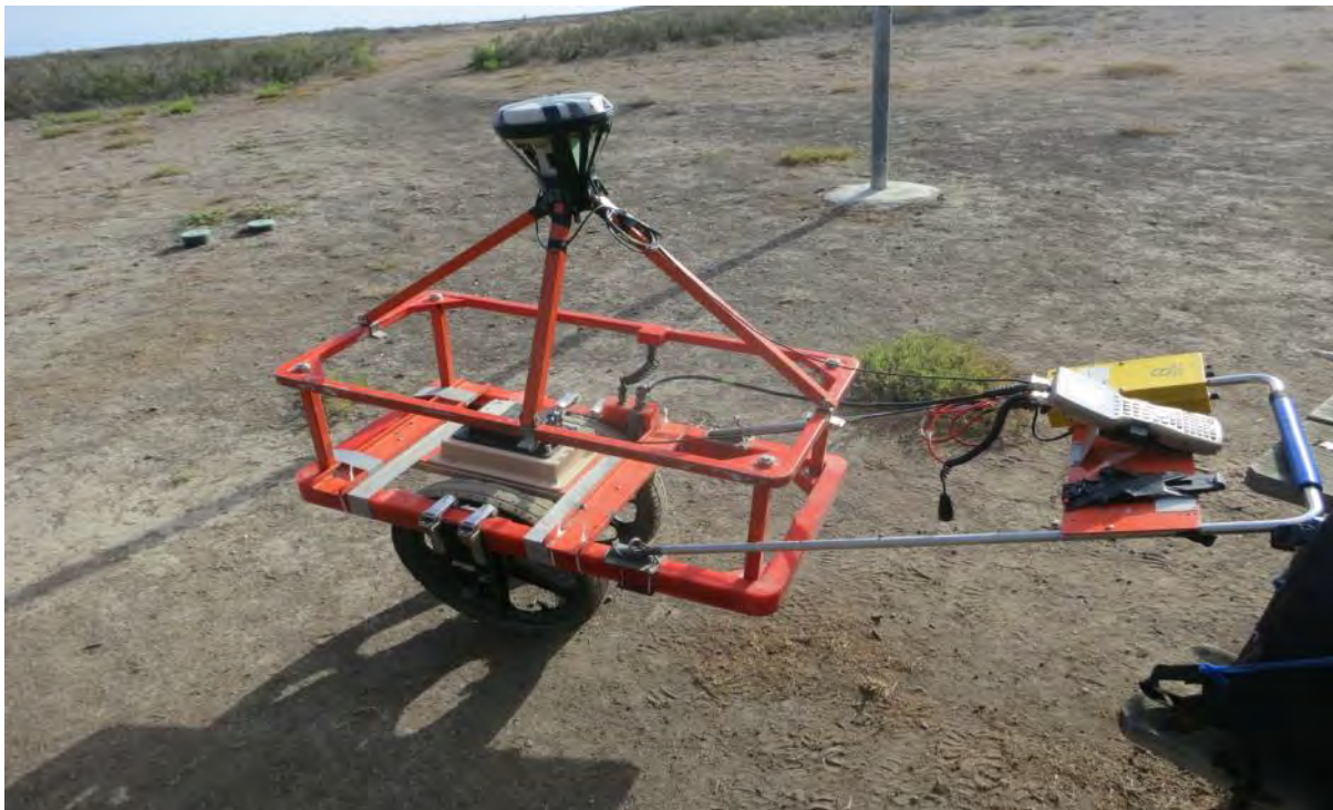
Photograph 20 EM61 modified for narrow trails
