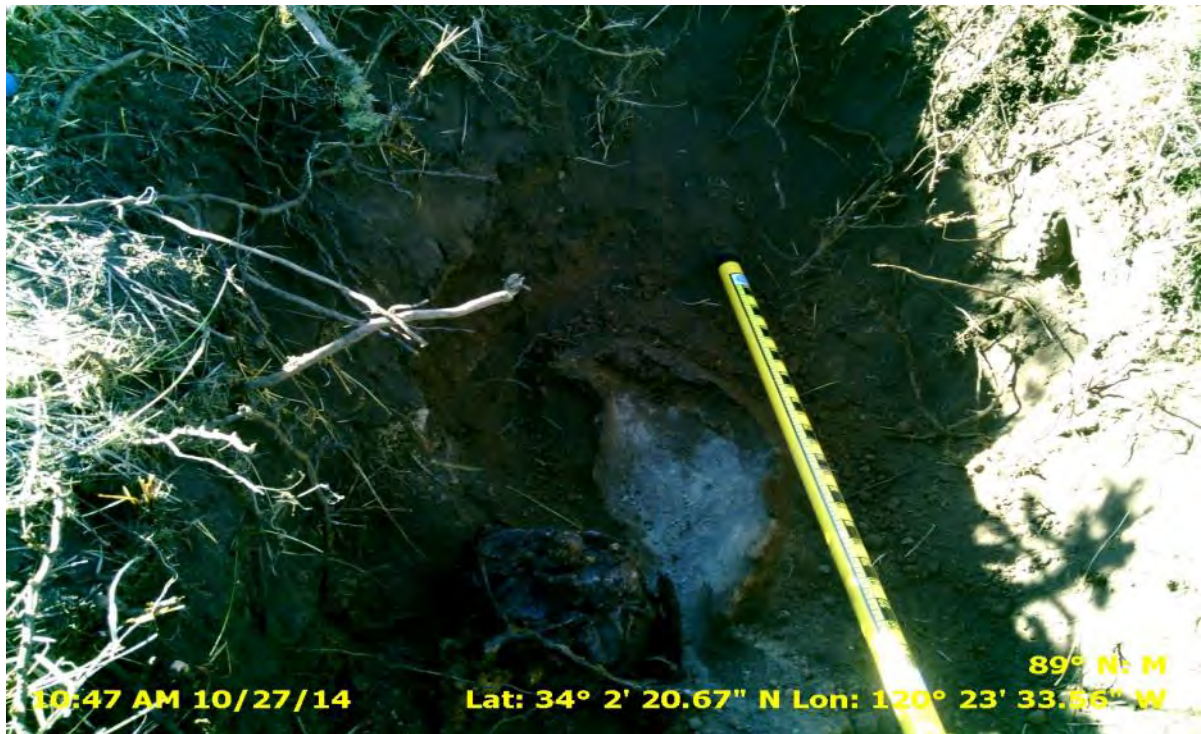
Photograph 38 Mk 15 100 lb practice bomb (left in place)
