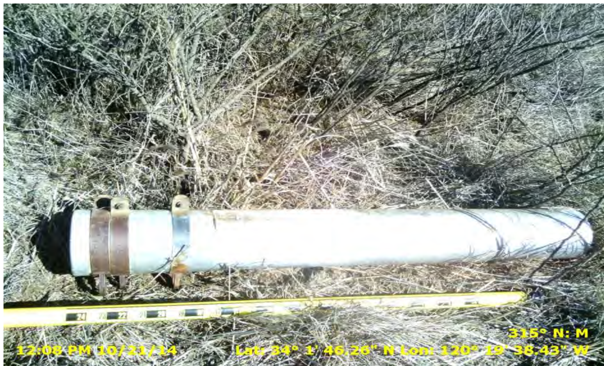
Photograph 40 Mk 25 flare canister
