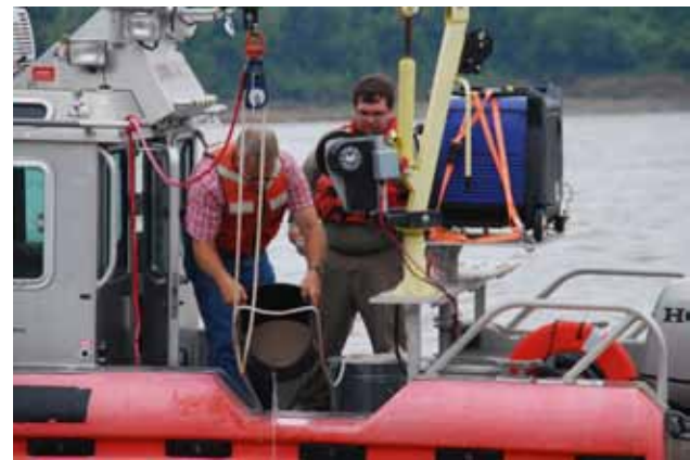
ABOVE: Thad Pratt of the Engineer Research and Development Center and Richie McComas of the Corps' Vicksburg District, pour off excess water from a river sediment sample prior to bagging and logging.
