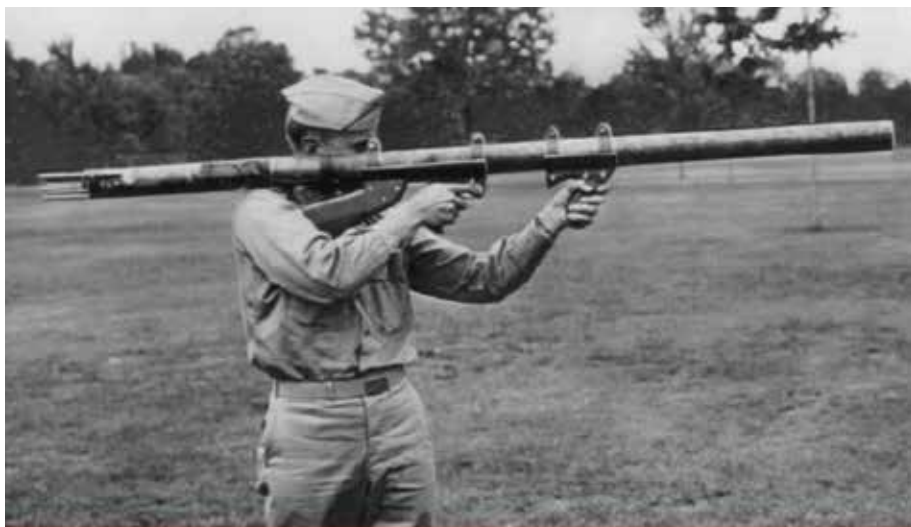
2d Lt. Edward G. Uhl demonstrates the first bazooka prototype. Cobbled together from a length of discarded pipe, a wooden rifle stock, and homemade hand grips, it outperformed the spigot mortars developed by munitions manufacturers. (National Archives)
