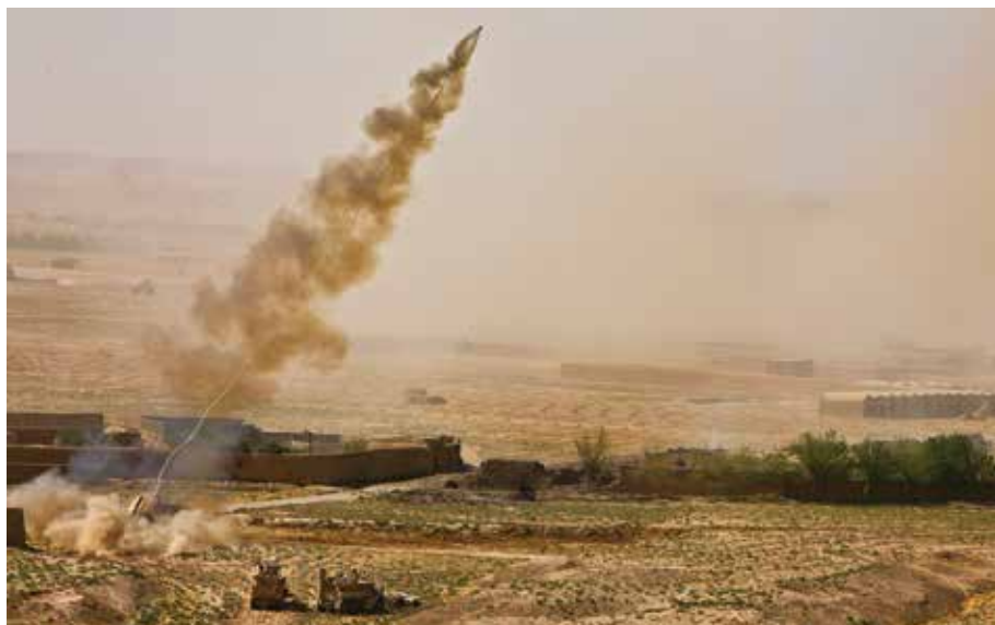
Assault Breacher Vehicle launching a mine-clearing line charge. (Photo by Cpl Jeff Drew.)
