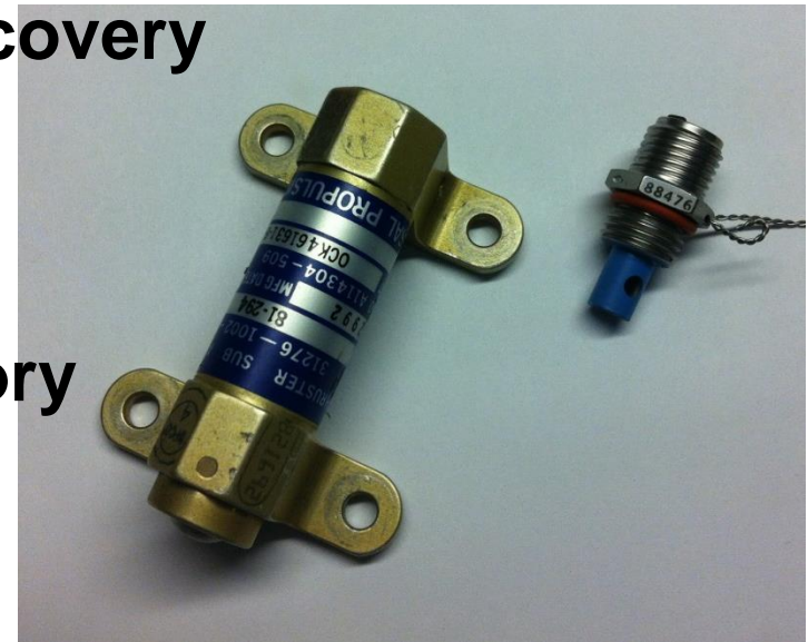
ACES II Harness Release Thruster and Cartridge
