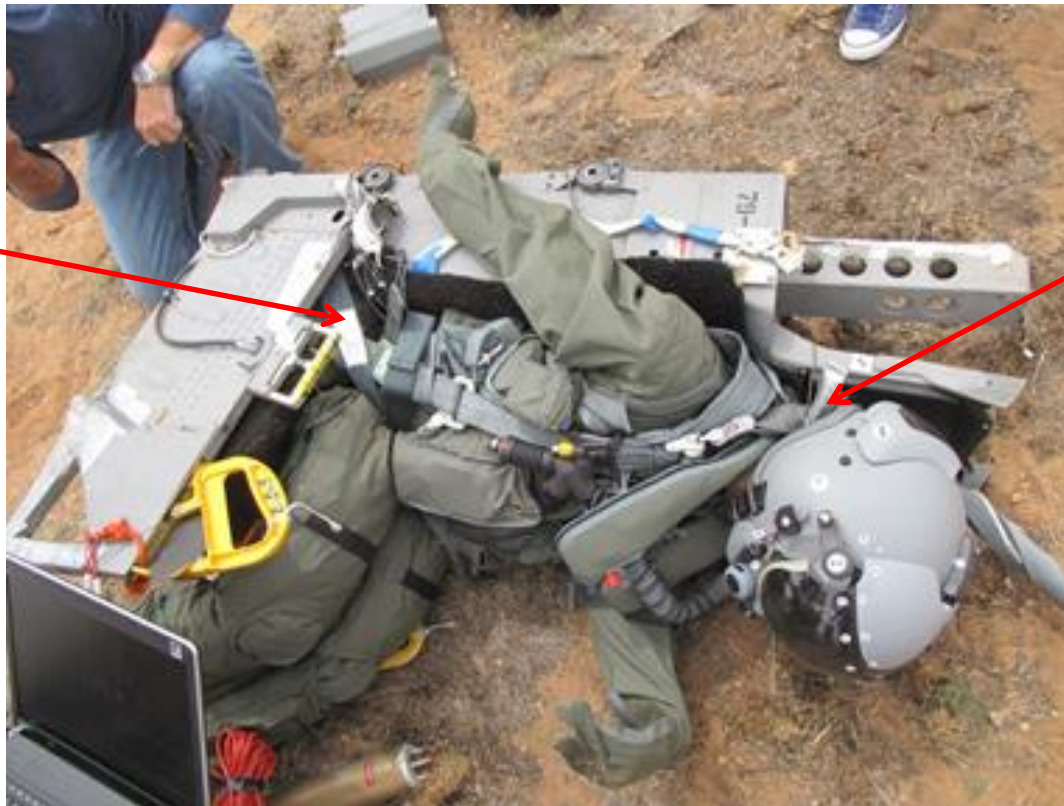
Manikin failed to release from seat
