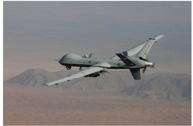
DARPA's research in the 1980s into long-endurance UAVs led to the development of the MQ-9 Reaper ISR and strike platform.
