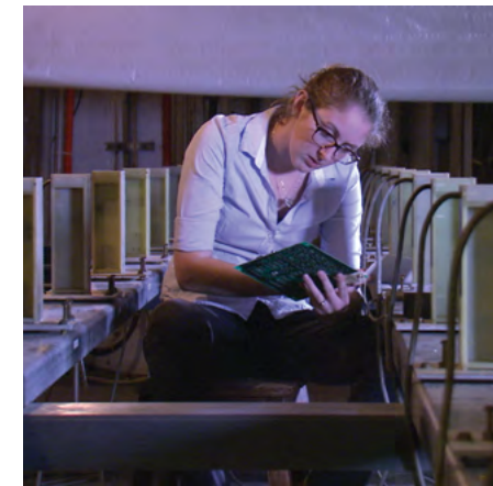
A physicist assigned to the Underwater Electromagnetic Signatures and Technology Division at the NSWC, Carderock Division, works on one of the over 300 triaxial magnetic field sensors permanently installed in the Magnetic Fields Laboratory.
