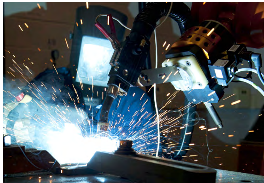
A robotic gas metal arc welder fabricates a weld in the robotic welding laboratory development system at Naval Surface Warfare Center, Carderock Division, in West Bethesda, Md. Carderock Division and their industry partners are developing highly specialized robotic welding systems to fabricate critical structures. The use of robotic automation improves worker safety, increases first-time quality, and reduces labor costs compared to traditional manual welding.
