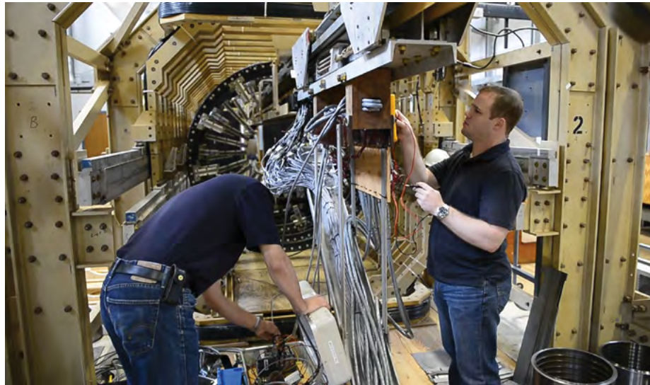
Engineers assigned to the Underwater Electromagnetic Signatures and Technology Division take measurements on the model track of the Magnetic Fields Laboratory. Photo by U.S. Navy
