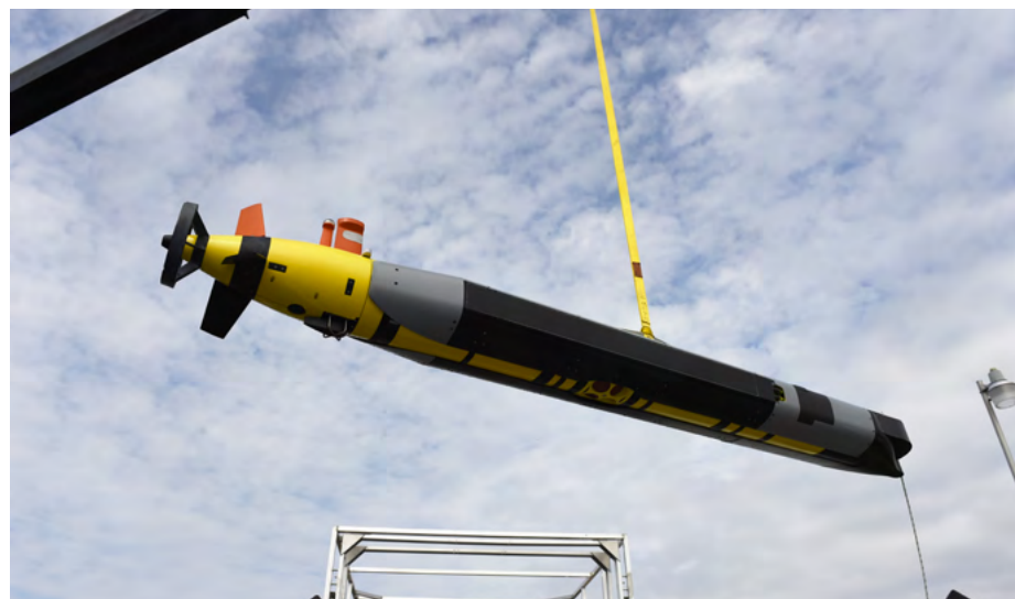
The Remus 600 is an example of the potential submarine payload relying on lithium-ion batteries for its energy source.
