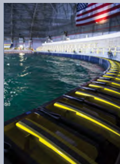
Close-up view of some of the 216 individually operated wavemaking paddles in the Maneuvering and Seakeeping basin at Naval Surface Warfare Center, Carderock Division.
