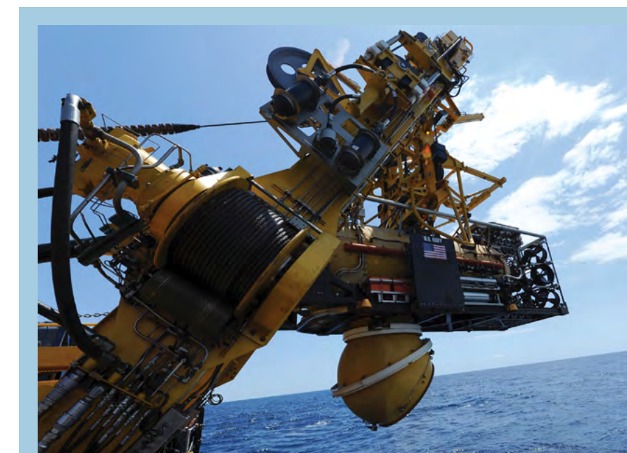
The Submarine Rescue Diving and Recompression System’s (SRDRS) Rescue Capable System (RCS), shown here in an exercise from 2011, is the U.S. Navy’s deep-submergence submarine rescue asset. The Naval Surface Warfare Center, Carderock Division, together with Portsmouth Naval Shipyard, played a key role in a time-sensitive recertification of the Pressurized Rescue Module, the pressure hull structural component of the SRDRS, in 2013. The team provided analytical evaluation and hydrostatic testing in Carderock’s Deep Submergence Test Facility in support of the recertification. Carderock expedited the testing necessary for the recertification, providing NAVSEA with the critical data 10 days ahead of schedule.
