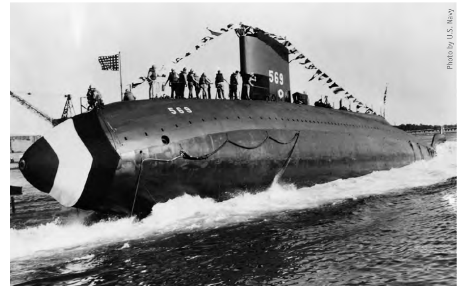
USS Albacore (AGSS-569) was a significant development in the design of submarines because of its hydrodynamic design developed at Carderock. With the advent of nuclear propulsion, sustained underwater operations allowed submarines to be built in a manner which embraced underwater hydrodynamics without having to perform well on the surface of the water.
