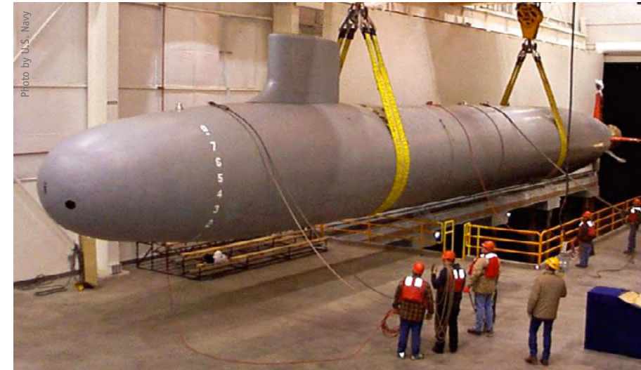
LSV 2 Cutthroat, the world's largest unmanned autonomous submarine, has been operating at the Acoustic Research Detachment in Bayview, Idaho, since its delivery in 2001. Cutthroat offers a cost effective and scalable research and development platform which enables advanced research and development in the areas of submarine hydroacoustics, hydrodynamics, and radiated noise reduction.
