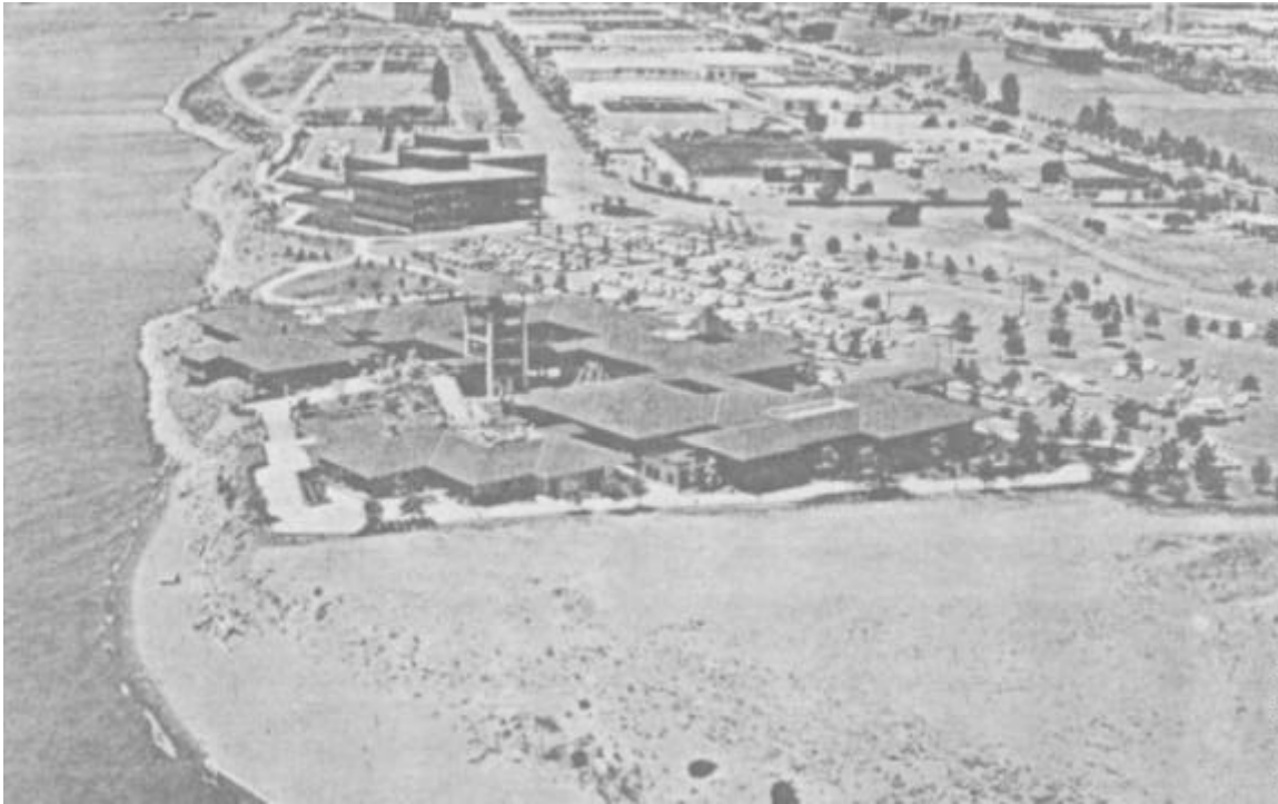
Figure 15-5. A large shopping mall, Port Center, was built on dredged material at Swan Island on the Columbia River at Portland, Oregon. It included shopping and commercial areas, as well as low-rise office buildings.
