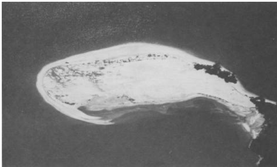
Figure 7-7. An addition built by Jacksonville District to Sunken Island in Hillsborough Bay, Florida, during maintenance dredging operations. It was built as seabird nesting habitat in cooperation with the National Audubon Society.
