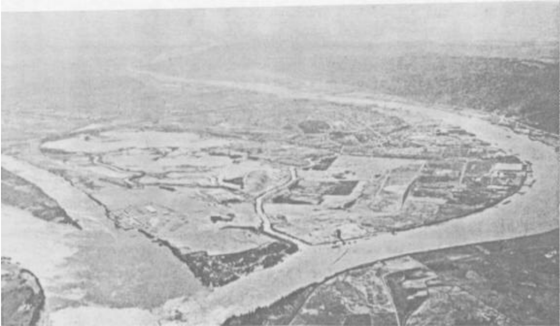
Figure 15-2. Two port facilities built on dredged material at Portland, Oregon, at the confluence of the Columbia and Willamette Rivers. A container port is located on the Columbia (left) and a grain terminal is located on the Willamette (right)
