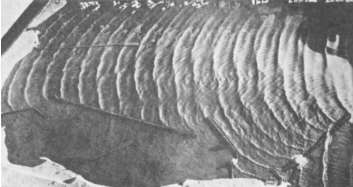
Figure 3-11. Model study for proposed harbor at Port San Luis, California. Note how proposed breakwaters attenuate waves from the South.
