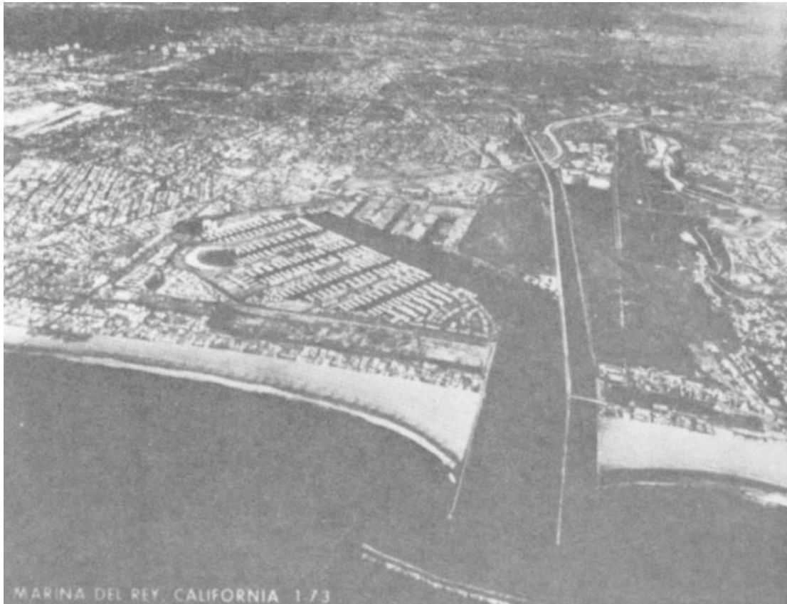
Figure 3-3. Separation of river flow from boat basin at Marina Del Ray, Los Angeles County, California.
