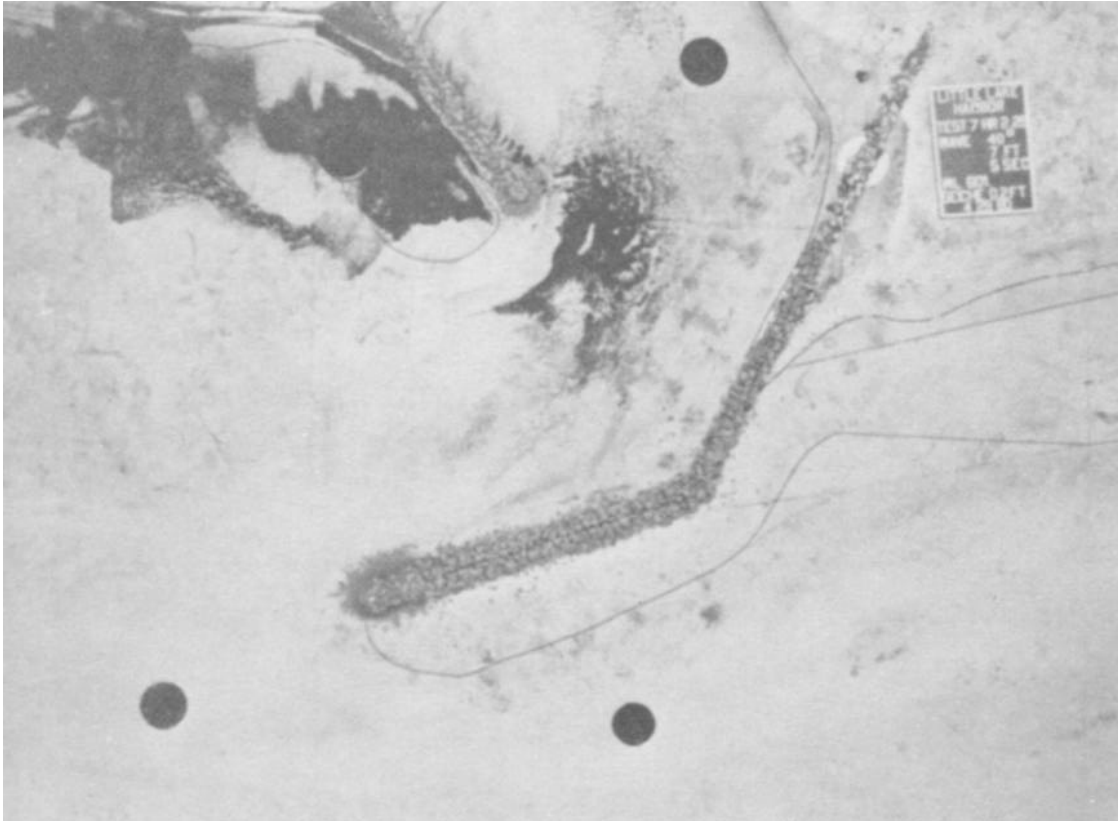
Figure A-24. Tracer deposits in the Little Lake Harbor model for base tests.
