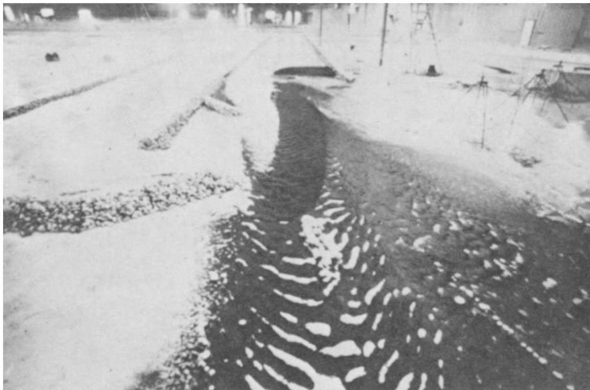
Figure A-19. Deposits at the entrance with the 400-foot-long diversion channel installed, Mission Bay Harbor model.
