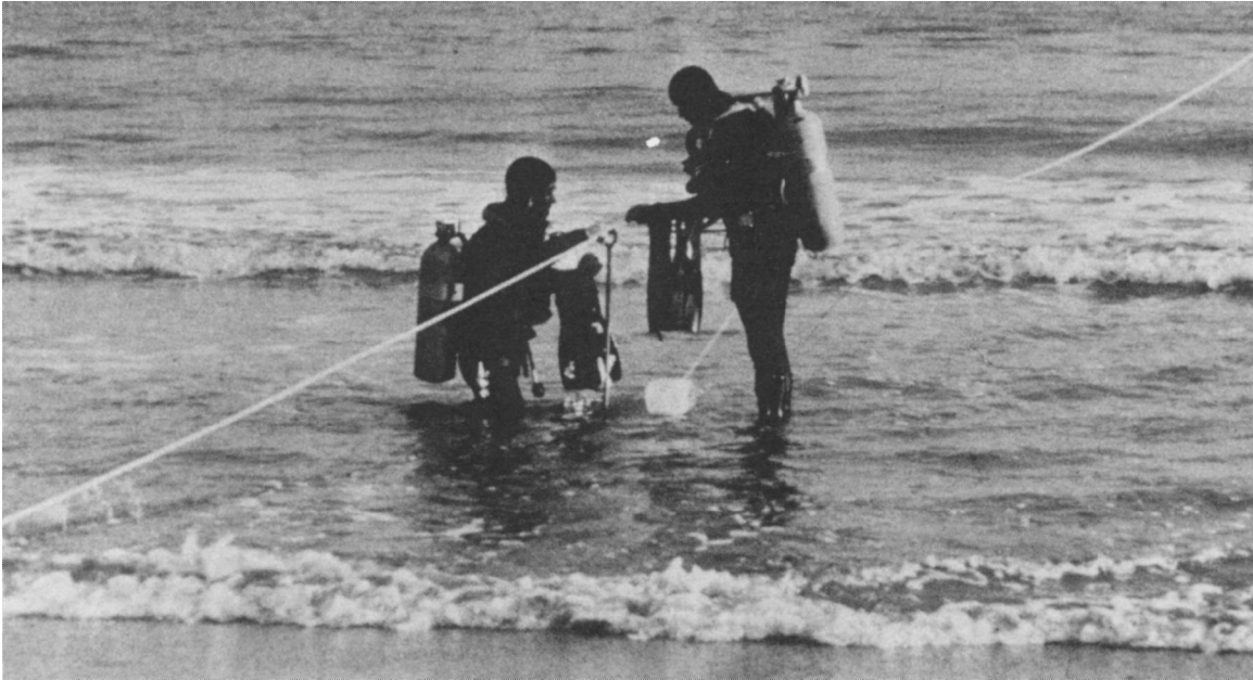
Figure 7-4. Diver using transect line in the surf
