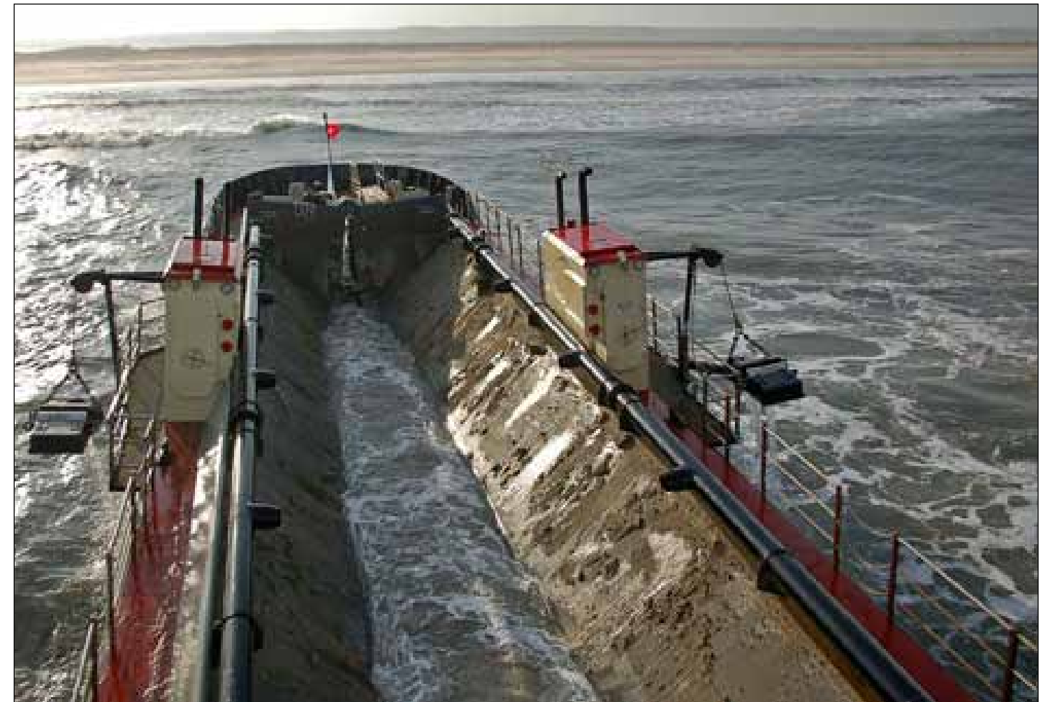
The Currituck pumps dredged material into its hull. (Photo by Hank Heusinkveld)
