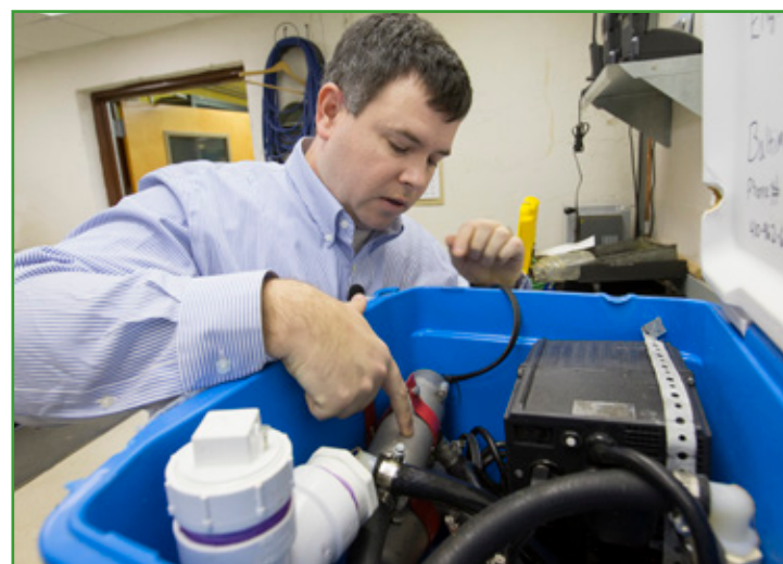
Baltimore District geologist Ethan Weikel points to the miniature heater in the ground-source heat pump system he developed. Weikel’s system, housed in a portable ice chest, gives engineers a more mobile and less costly way to measure the heat transfer capabilities in the earth. (Photo by Jhi Scott)
